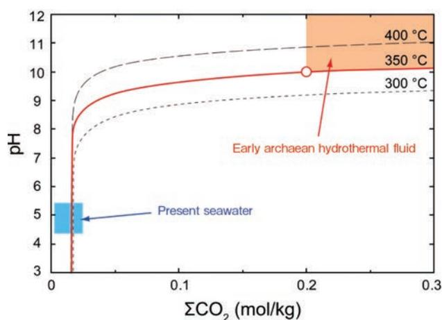
Figure 1. Relationship between the  $\text{CO}_2$  concentration and pH in hydrothermal fluid.
