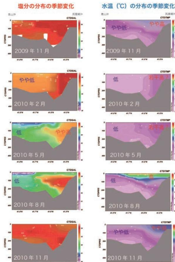
Figure 8. Cross-sectional distribution of salinity (left row) and temperature (right row) observed in the eastern Tsugaru strait. From top, cross-sectional distributions in November 2009, February, May, August, and November 2010.
