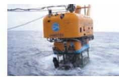
7,000 m Class Remotely operated vehicle
