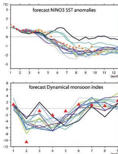
Figure 7. 2010 prediction results, with 4D-Var coupled atmosphere-ocean reanalysis as initial values. Monthly time-series of (top) the El Niño Index (sea surface water temperature deviation in the Niño 3 region) and (bottom) the Dynamical Indian Monsoon Index. Broken lines show results of respective ensemble experiments; circles and triangles show observed values.
