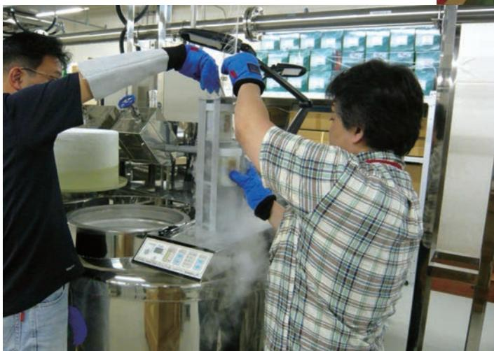
Figure 9. RMS being lowered into the special freezer tank (set to  $-160^{\circ}\text{C}$ ) for storage.
