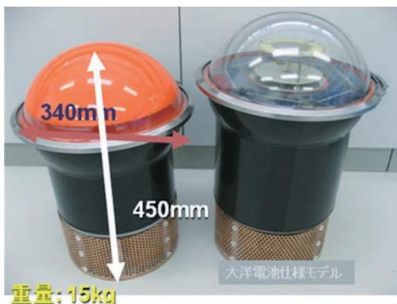
Figure 4. Appearance of the drifting carbon dioxide sensors developed at MIO. Left: ordinary use type; Right: solar cell-equipped type.
