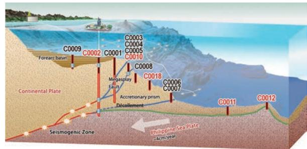
Figure 2. Outline diagram of the Nankai Trough Seismogenic Zone Drilling Plan
