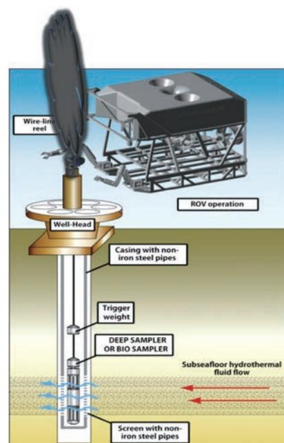
Figure 8. Conceptual diagram of the artificial hydrothermal vent
