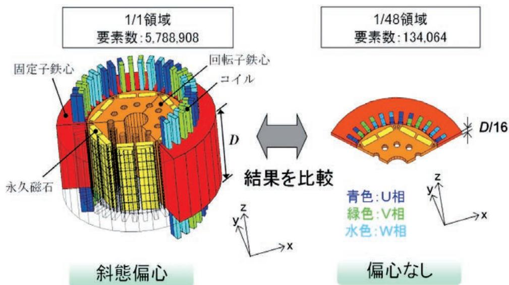
Figure 8. An analysis model of an IPM motor.
