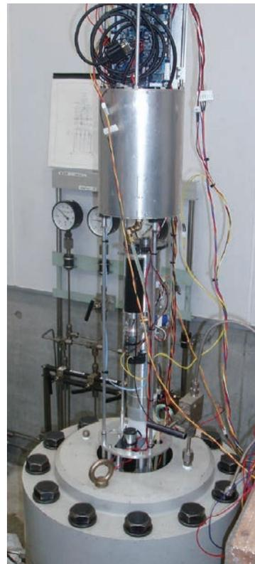
Figure 6. Deep NINJA prototype being tested (photo provided by Tsurumi-Seiki Co. Ltd.).
