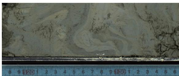
Figure 4. Deformed structure inside submarine landslide mass (at 139 m below the seafloor, 3084 m deep)
