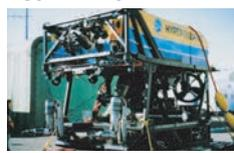
3,000 m Class Remotely operated vehicle
