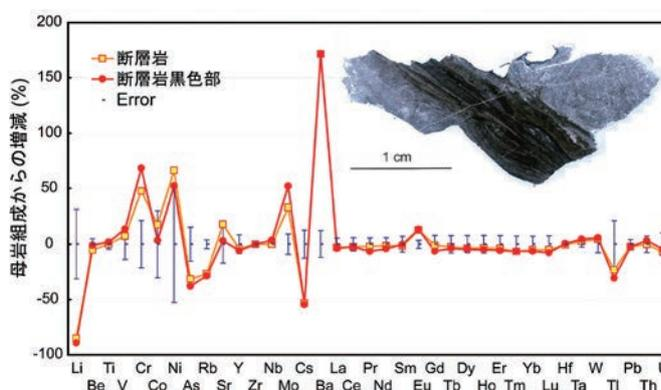
Figure 4. Microscope image and the results of analysis of fault rock in the Emi accretionary prism in Boso Peninsula. Decreases in lithium (Li) and cesium (Cs) indicate the generation of hot water at temperatures of 350°C or higher during the earthquake. A similar event may occur in the current Nankai accretionary prism.
