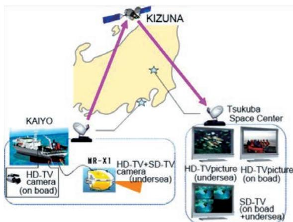
Figure 3. Transmitting HDTV test pictures via satellite.
