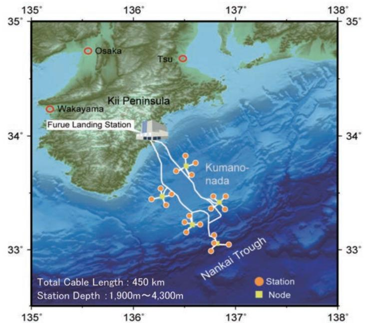
Figure 1. Deployment diagram of the Dense Ocean-floor Network System for Earthquakes and Tsunamis (DONET).
