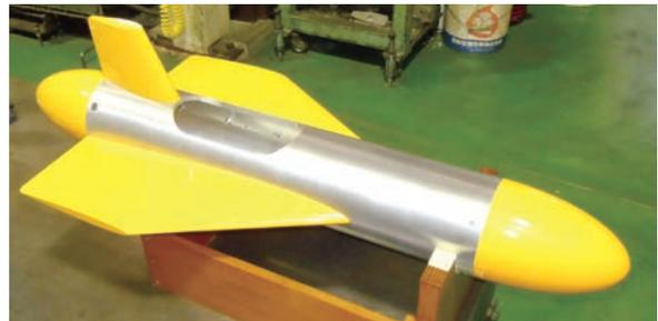
Figure 5. Model of the shuttle-type robotic vehicle.
