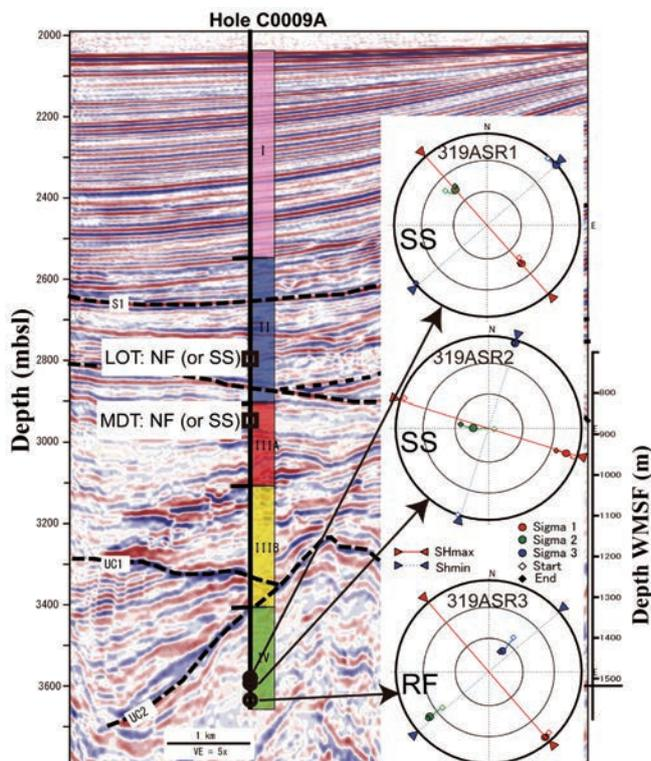
Figure 2. Measurement of anelastic strain recovery (ASR) using the core samples collected by the drilling of Site C0009A located immediately above the massive earthquake zone in the Nankai Trough indicated that the stress conditions were different in the cover sediment and the accretionary prism (Fig. 2; Lin et al., 2010, AGU).
