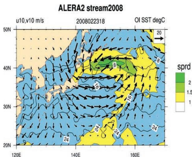
Figure 7. Wind velocity at 10 m above ground (m/s, arrow), its error (m/s, color) and the sea surface temperature (°C, contour) at 18:00 UTC on February 23, 2008 (3:00 Japan time on February 24).
