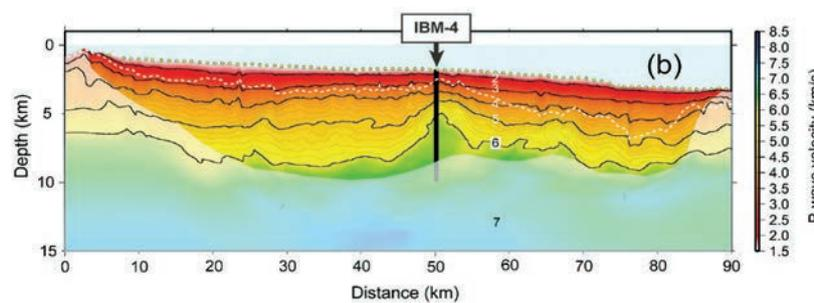
Figure 10. Crustal structure of the east-west profile line transecting IBM4. IBM4 is an island arc volcano of the Eocene-Oligocene Epoch under which the middle crust is seen protruding into the shallow layer, indicating that it is the most suitable drilling point to uncover the relationship between island arc volcanoes and the middle crust.
