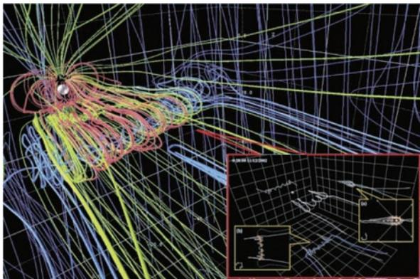
Figure 5. A visualization result of magnetic field lines calculated by the global magnetospheric magnetohydrodynamic (MHD) simulation. Distinctive magnetic field lines which affect the magnetospheric dynamics are automatically extracted and classified according to their three-dimensional topologies, by a visual data mining technique which is a typical technique of smart visualization.
