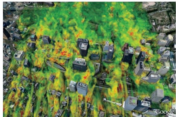
Figure 2. Three-dimensional temperature distribution in a simulation by MSSG with a 5-m horizontal resolution of the conditions of the atmosphere on the periphery of Yuraku-cho, Tokyo, at 15:00 on August 5, 2005. It is expected to be applied for elucidation of the mechanism of the heat-island phenomena, proposals on adaptive measures for cooling urban areas, and quantitative evaluation of effects.
