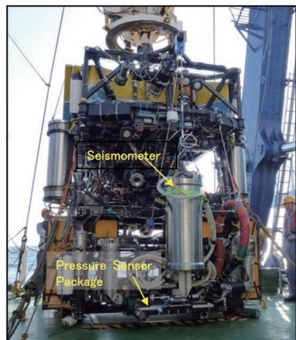
Figure 2. The *Hyper-Dolphin*, an unmanned operated vehicle modified to install observation equipment on the seafloor.
