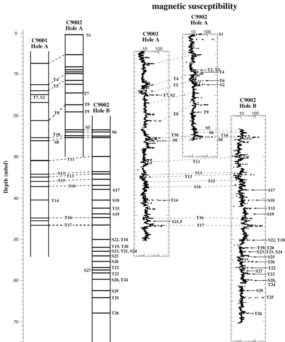
Fig. 15 Inter-hole correlation of lithology and magnetic susceptibility. Solid horizontal lines in the left columns indicate the tephra (numbered as T1, T2, ...) and sand / sandy clay (numbered as S1, S2,...) horizons.
