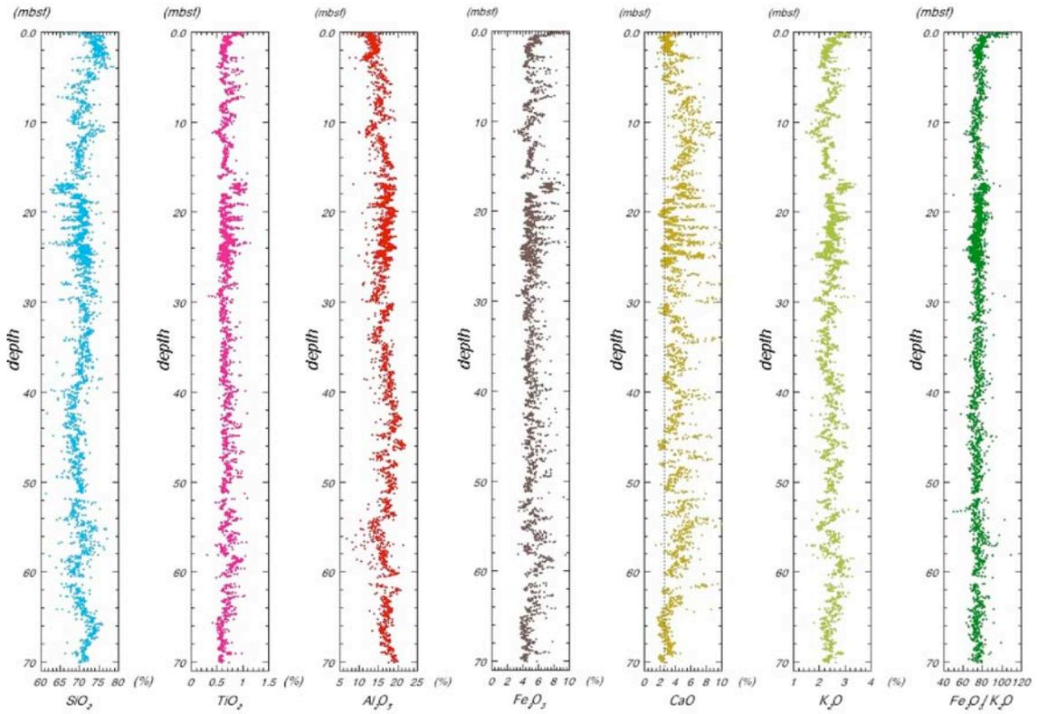
Fig. 12 XRFCL results plots of C9002A-B after data exclusion and normalization. Variations of each profile become clearer and dispersion is reduced. Relatively constant ratio of iron and titanium means that heavy mineral composition is essentially invariant. In calcium profile, which has a base concentration, the variations are probably generated by calcareous microfossil population changing.
