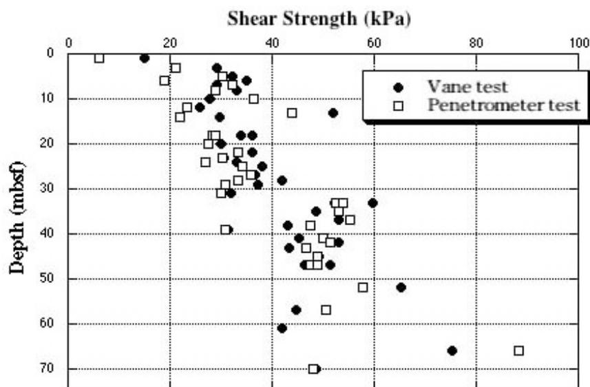
Fig. 9 Plot showing the result of shear strength test
