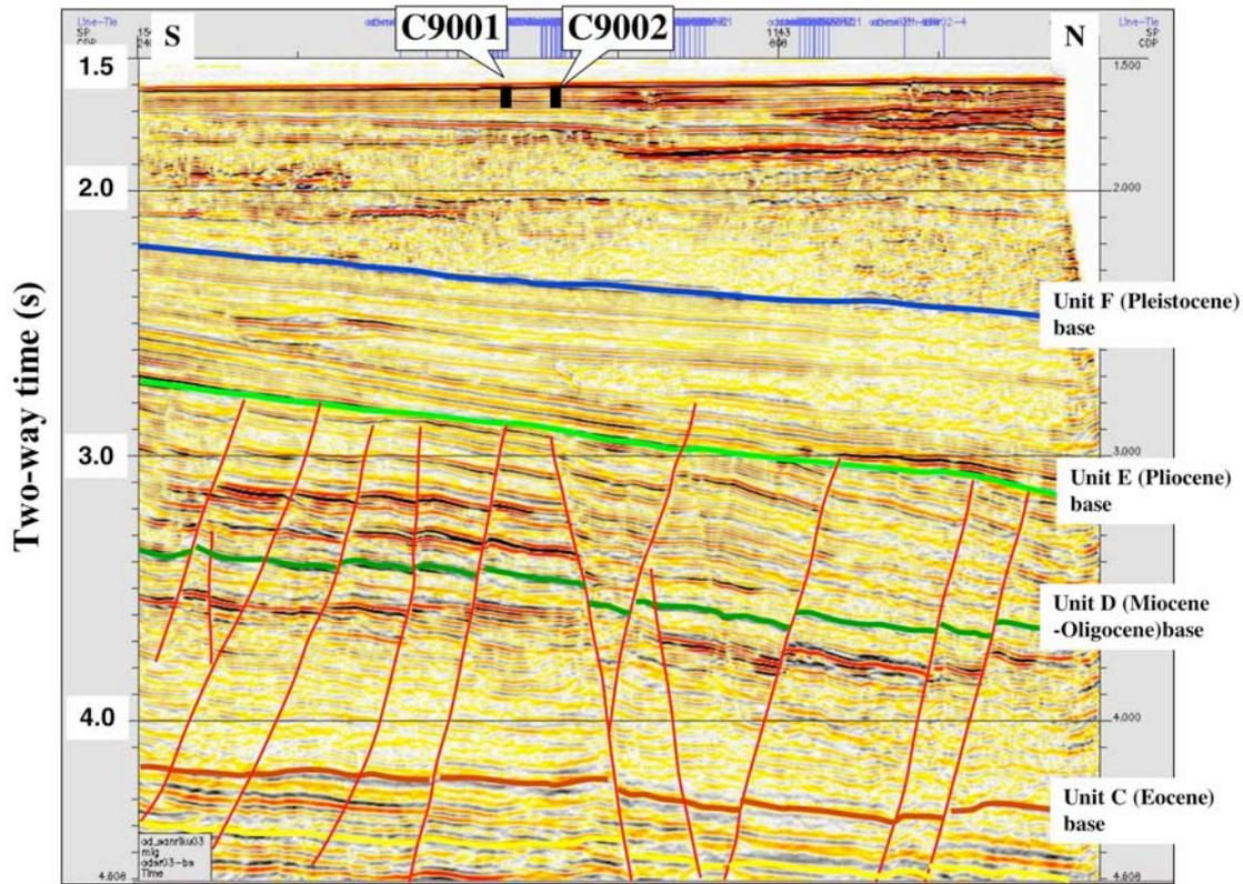
Fig. 2 N-S seismic cross-section along ODSR03–BS (line location is shown in Fig. 1). Drill sites C9001 and C9002 are also shown. Data acquisition was by *R/V Polar Princess* in 2003. Geologic interpretations are done by A. Ibusuki (unpublished data).
