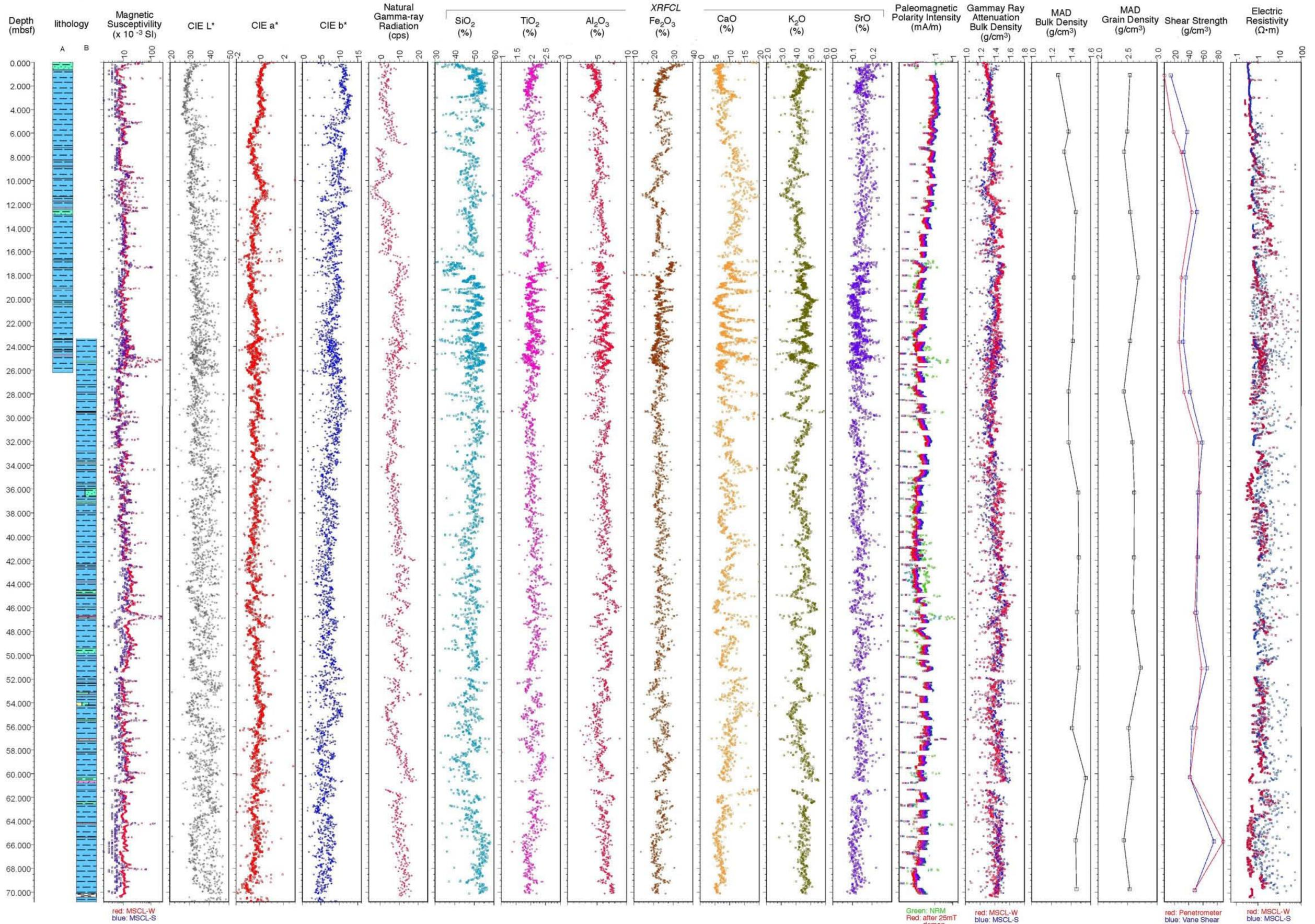
Fig. 7 Synthesized columnar profiles of physical, chemical and magnetic properties and lithology for Site C9002 Hole A and B. All data for each profile within the plot range are shown without any filtering. Equally spaced spikes like "brush" in some profiles, especially in paleomagnetic intensity, are corresponding to section boundaries. All graphs are created by using Composite Log Viewer, J-CORES.
