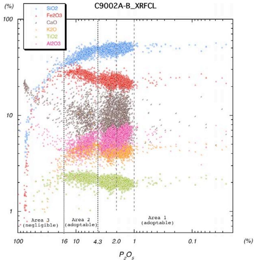
Fig. 11 Variations of  $\text{SiO}_2$ ,  $\text{TiO}_2$ ,  $\text{Al}_2\text{O}_3$ ,  $\text{Fe}_2\text{O}_3$ ,  $\text{CaO}$  and  $\text{K}_2\text{O}$  versus  $\text{P}_2\text{O}_5$ . Overestimation in phosphorus can be used as an indicator of poorly quantified data. Data of a horizon where phosphorus content is given lower than 16 % can be neglected.
