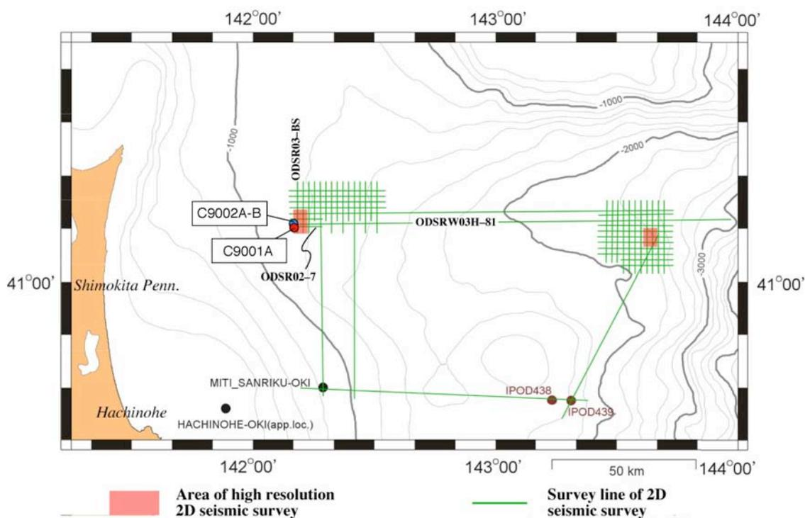
Fig. 1 Bathymetry map showing the drilling sites and survey lines of two-dimensional seismic survey
