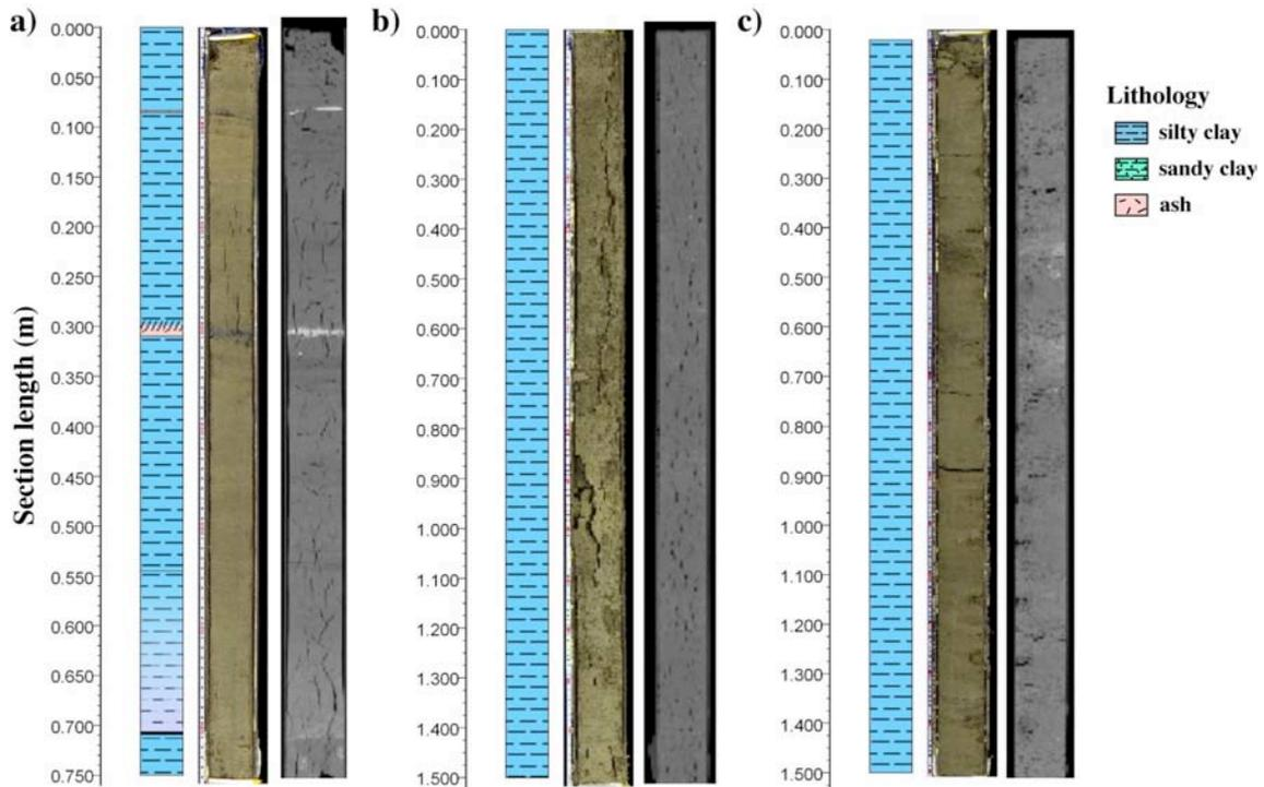
Fig. 5 Comparison of visual and CT images. a) Site C9001 Hole A Core 2 Section 1, b) C9001 Hole A Core 2 Section 3, c) Site C9001 Hole A Core 4 Section 4.
