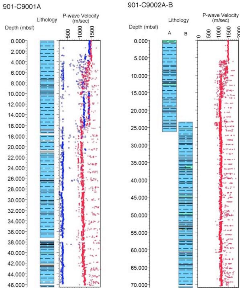
Fig. 8 Columnar profiles for P-wave velocity of Site C9001 Hole A and C9002 Hole A-B. Red open circle: MSCL-W, blue open square: MSCL-S (data of C9002 are not shown). All data for each profile within the plot range are shown without any filtering. Data like "brush" are corresponding to section boundaries.
