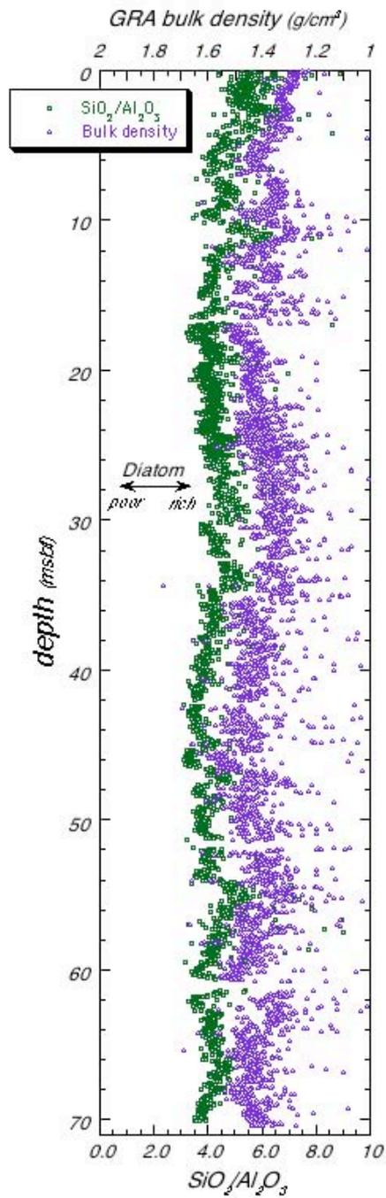
Fig. 13 Comparison of SiO<sub>2</sub>/Al<sub>2</sub>O<sub>3</sub> and bulk density of C9002A-B. Higher Si/Al reflects higher diatom population and bulk density of the sediments may be controlled essentially by diatom concentration.
