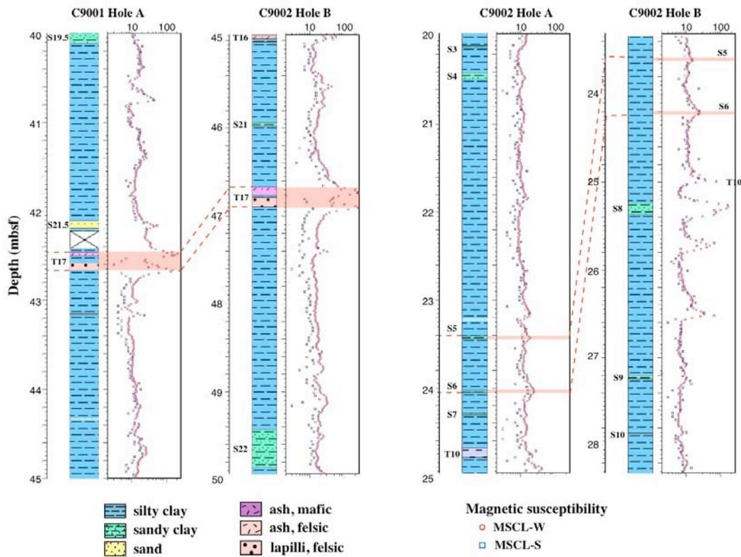
Fig. 14 Inter-hole depth correlation between Site C9001 Hole A and Site C9002 Hole B, and Site C9002 Hole A and Site C9002 Hole B.
