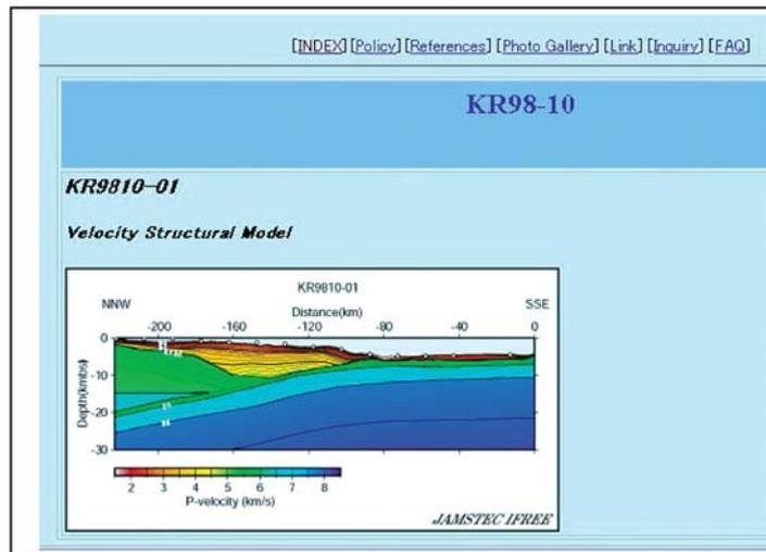
Figure 5: An example of the P-wave seismic velocity model along the KR9810-01 line. The color index shows the P-wave velocity contrast.
