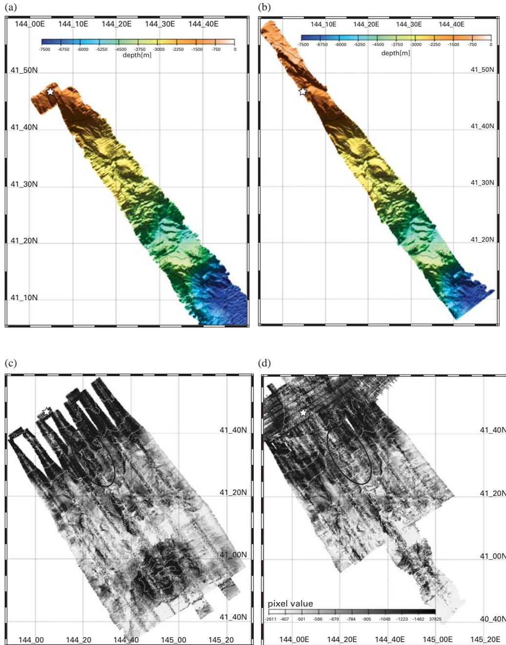
Figure 8: (a) Corridor bathymetry image of the three years before the 2003 Off-Tokachi Earthquake. (b) Corridor bathymetry image of the three months after this earthquake. (c) Backscattering image of the three years before the earthquake. (d) Backscattering image of the three months after the earthquake. White asterisks denote the epicenter of the earthquake.
