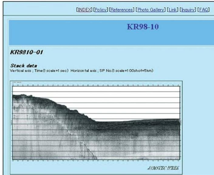
Figure 4: An example of the MCS section along the KR9810-01 line. The displayed MCS sections are combined to perform a time-migrated analysis. The descriptions are as follows:
