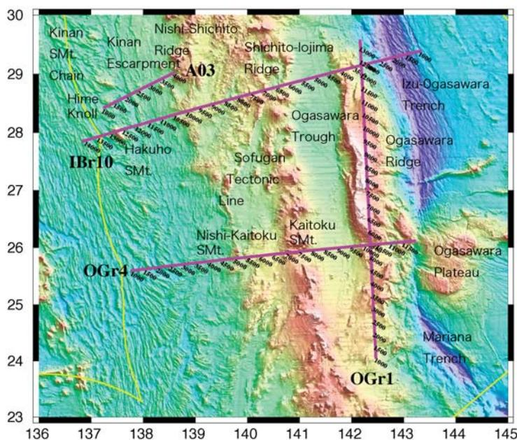
Figure 1: Map of the experimental area. Thick magenta lines show MCS lines. Labeled numbers represent the field shot point number.
