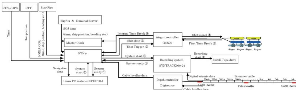
Figure 3: MCS recording system of R/V Kairei. Circled numerals show the signal transfer flow in the system.
