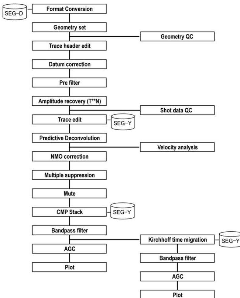
Figure 4: Flow chart of on-board processing of MCS data.
