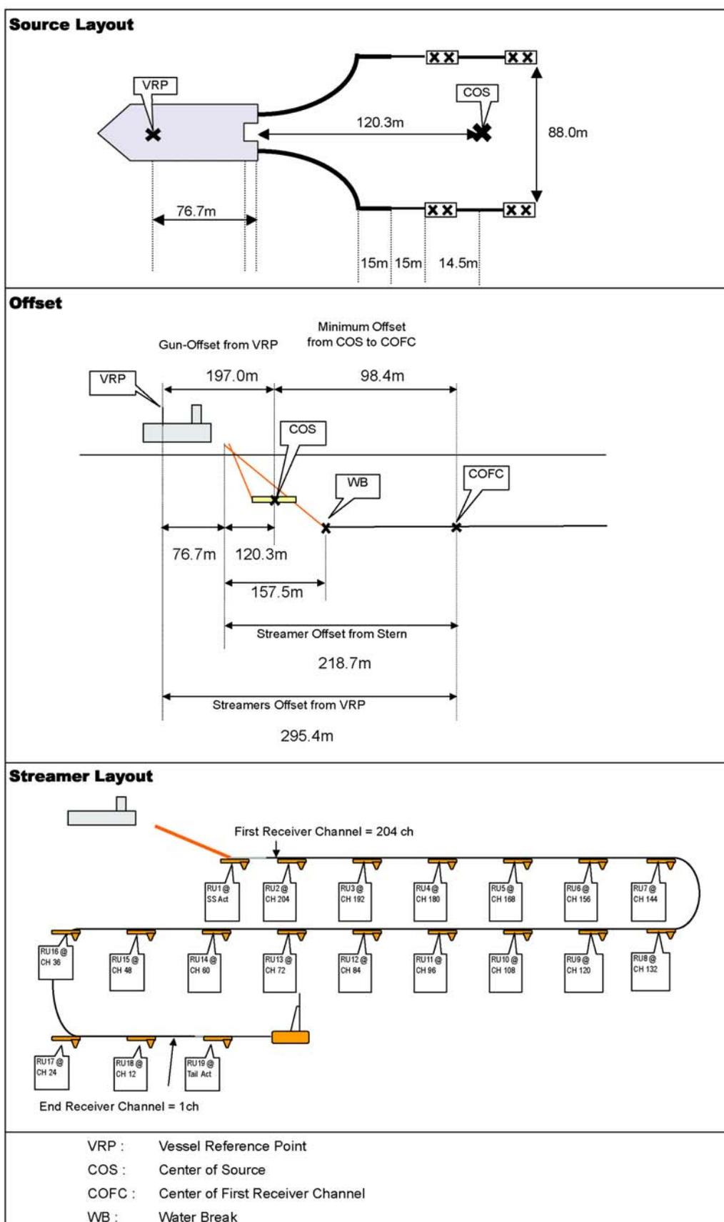
Figure 2: Geometry of the airgun system and the hydrophone streamer.
