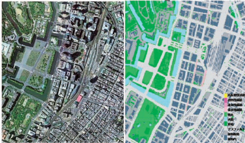
Fig. 3-12. Left: simulation area picture taken by a aircraft, Right: distribution obtained land use data for whole of simulated area. Boundary data out of those simulations area is interpolated from meteorological data (MSM) provided from Japan Meteorological Business Support Center.
