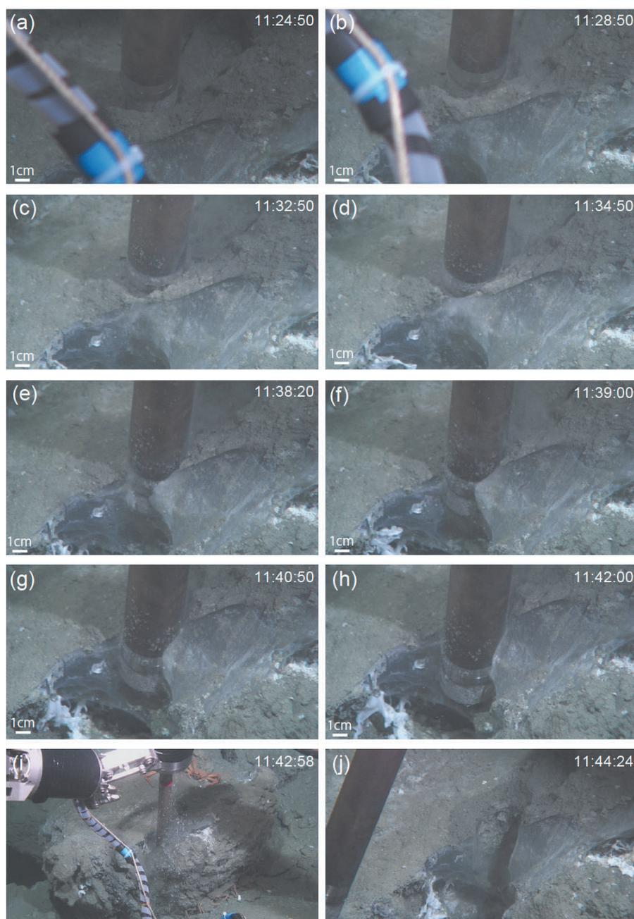
Fig. 7. Photos of dissolving methane hydrate by exposure to Heat sonde (preset temperature: 80°C). Methane hydrate was dissolved at 0.4 cm/min.
