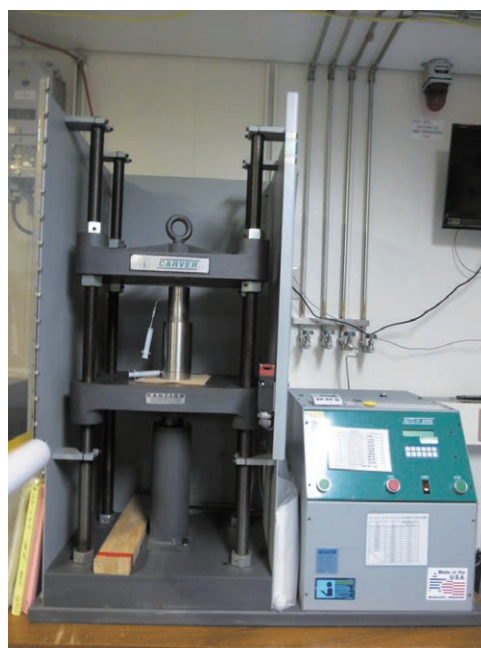
Fig. 1. Interstitial water squeezing system in Chikyu laboratory. The system is composed of a squeezer jacket in an automatic press machine.
