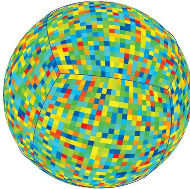
**Fig. 1** The SEM uses a mesh of hexahedral finite elements on which the wave field is interpolated by high-degree Lagrange polynomials on Gauss-Lobatto-Legendre (GLL) integration points. This figure shows a global view of the mesh at the surface, illustrating that each of the six sides of the so-called ‘cubed sphere’ mesh is divided into  $26 \times 26$  slices, shown here with different colors, for a total of 4056 slices (i.e., one slice per processor).
