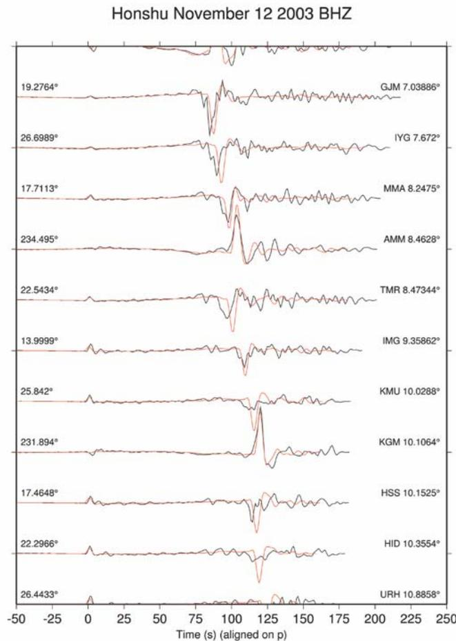
**Fig. 4** Broadband data and synthetic displacement seismograms for the 2003 South of Honshu earthquake, bandpass-filtered with a two-pass four-pole Butterworth filter between periods of 3.5 and 150 seconds. Vertical component data (black) and synthetic (red) displacement seismograms aligned on the arrival time of the P wave are shown. For each set of seismograms the azimuth is printed above the records to the left, and the station name and epicentral distance are printed to the right.
