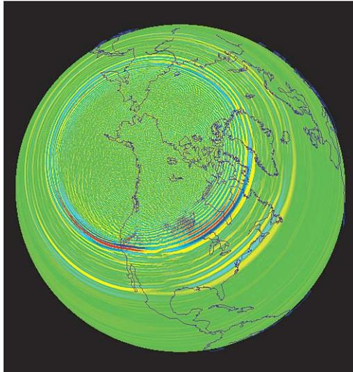
**Fig. 6** Snapshot of the propagation of seismic waves in the Earth during the November 3, 2002 Denali fault earthquake simulated in Tsuboi et al (2003). Note that large amplification in the western coast of the United States due to the source directivity is modeled well in the simulation.
