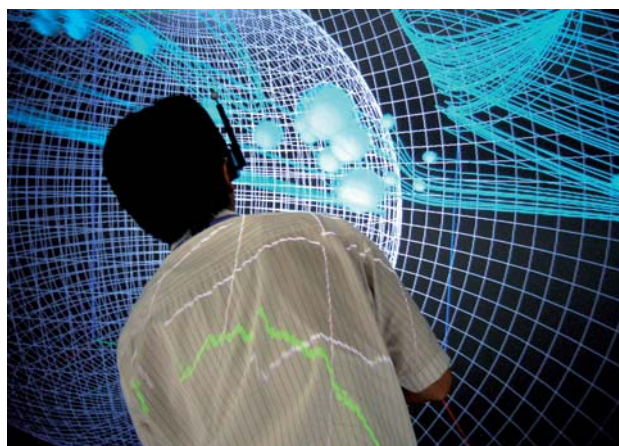
Fig. 8 The interactive data analysis of geodynamo simulation in the CAVE's VR space by VFIVE. "Particle tracer" method is used.
