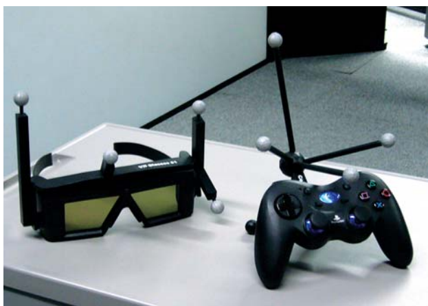
Fig. 7 The liquid crystal shutter glasses and the wireless controller with sets of markers for the optical positioning sensor system.
