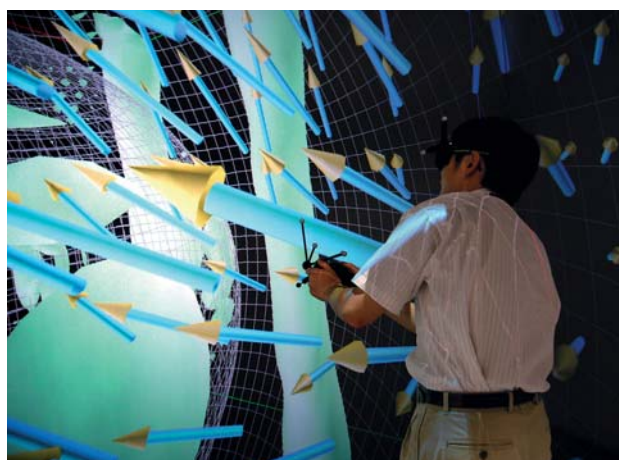
Fig. 9 The interactive data analysis of geodynamo simulation in the CAVE's VR space by VFIVE. "Local arrows" and "isosurface" methods are used.
