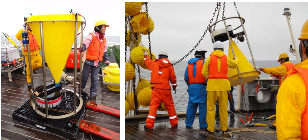
Fig.2.1.3-2. Recovered sediment trap moored at 1000 m (left) and that at 4800 m (right).
