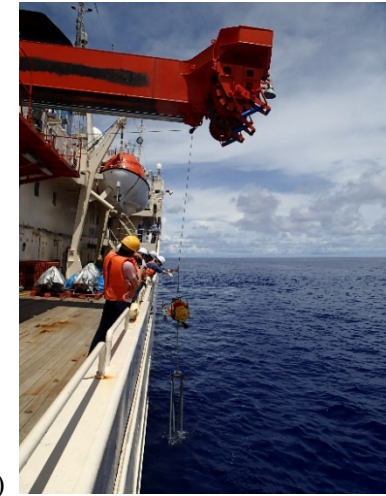
Photo 5-1. (a) OBEM JM6 on sea surface at O23. (b) OBEM VTM1 recovered in the night at O16. (c) OBEM ERI8 hooked by a crew at O08. (d) OBEM ERI14 lifted using the A-frame at O14. (e) OBEM JM106 lifted using the stretch beam at O15.
