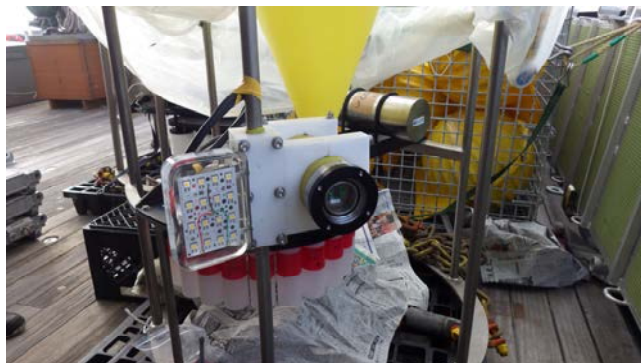
Photo 1. Underwater video camera on 1800 m sediment trap
