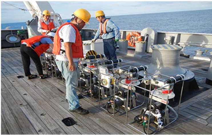
Photo: backscatter meters on water sampling system (upper panel), backscatter meters and underwater video camera on in situ pumping system (lower panel).
