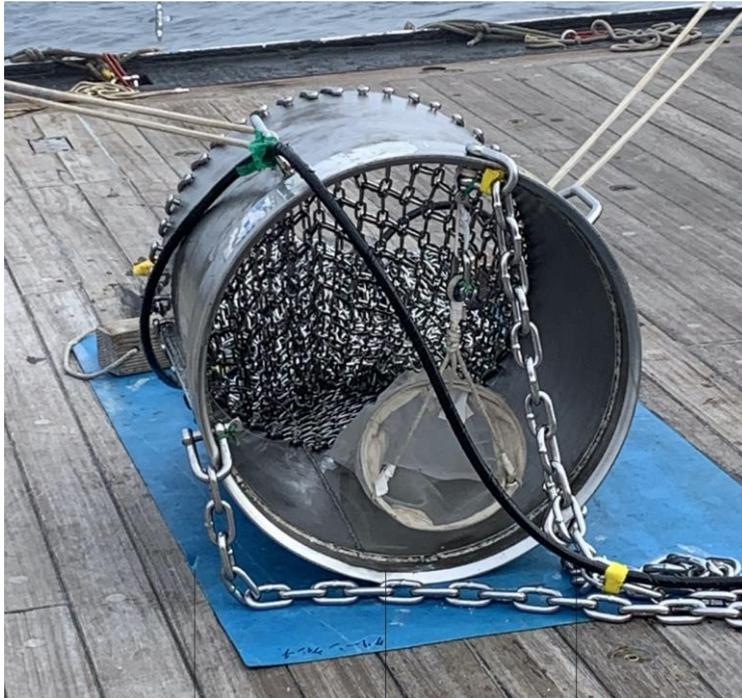
**Figure 3-4-4.** Nylon mesh bag installed in the barrel-type dredge for benthos sampling (D01).
