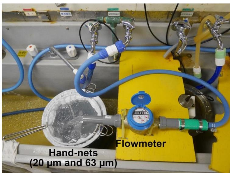
**Fig. 3-6-1.** Living plankton sampling system comprising the special hand-nets ( $20\ \mu\text{m}$  and  $63\ \mu\text{m}$  opening) and the flowmeter.
