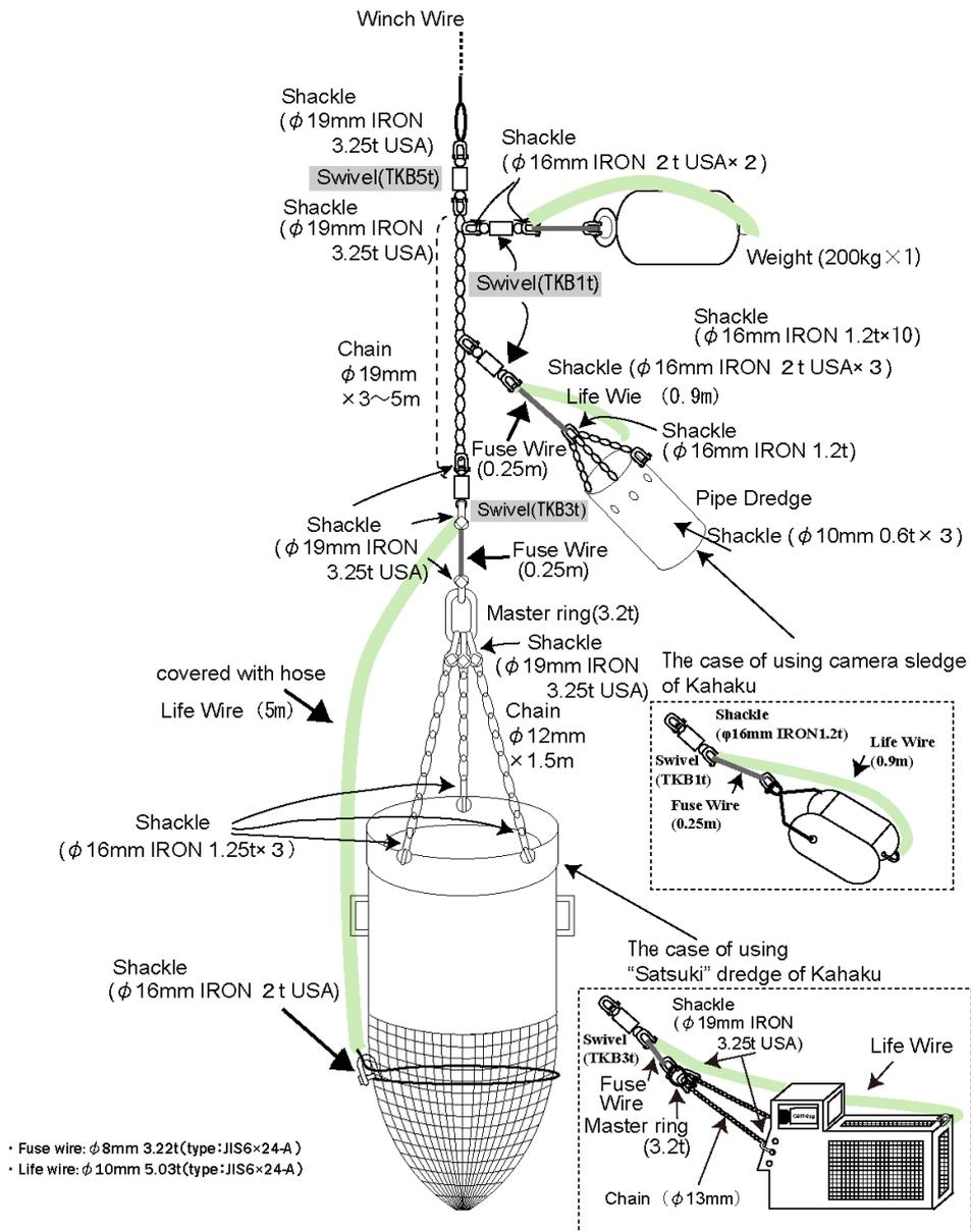
Figure 3-4-3. Detailed assembly of dredge systems used in KH-19-6-Leg 4 cruise.
