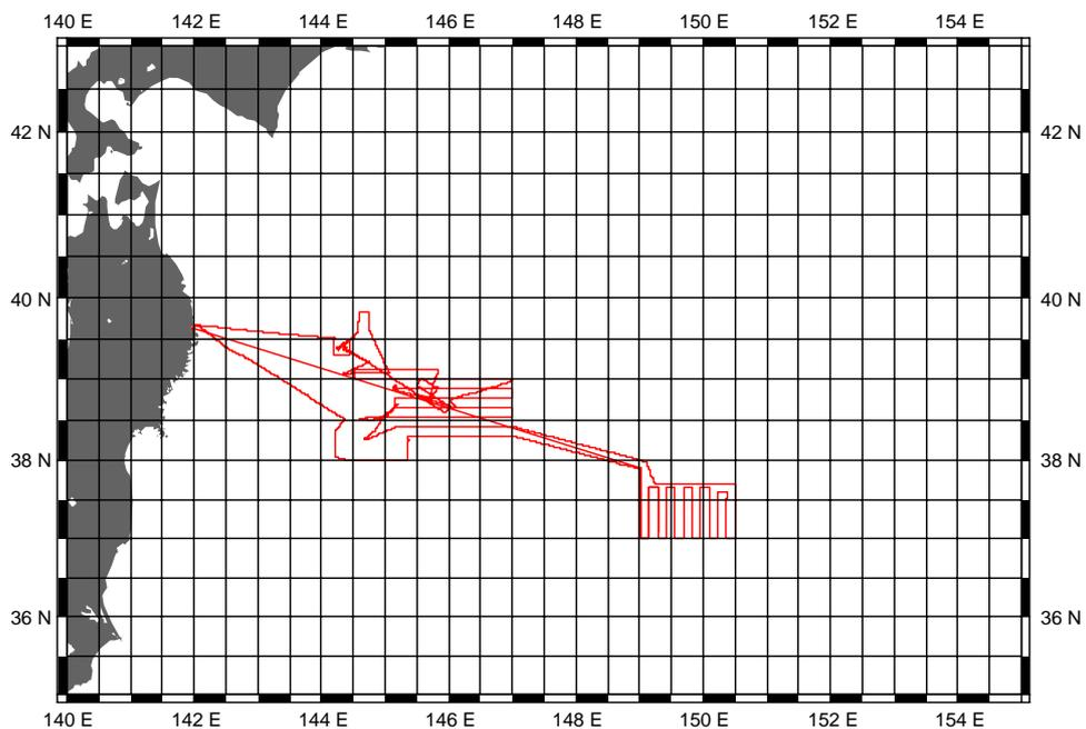
*Fig. 5-3: Track chart of seabeam survey. This image file is in this CD-ROM/ shiplog/ KR0307.ps*
