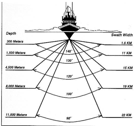
*Fig. 5-2: Schematic illustration of swath bathymetric survey.*
