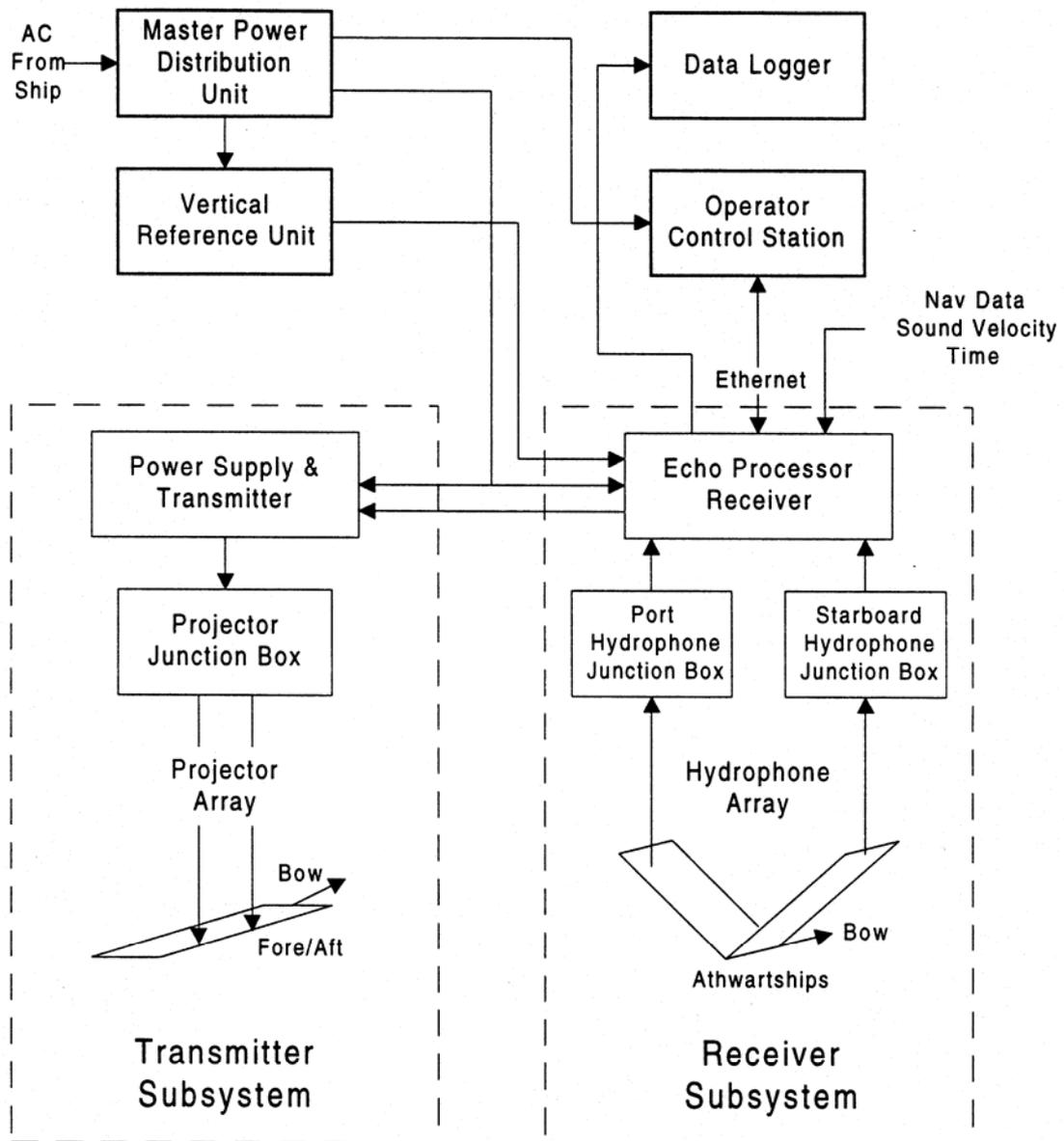
Fig. 5-1: Basic diagram of the SAE BEAM system.. Details are described in the text.
