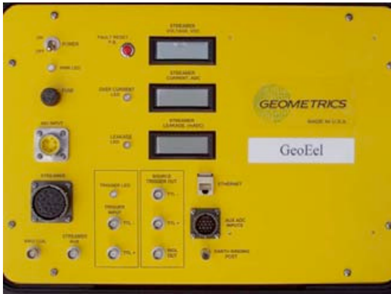
SPSU (Streamer Power Supply Unit. Provides interface connections between computer, gun controller, power, and other connections.
