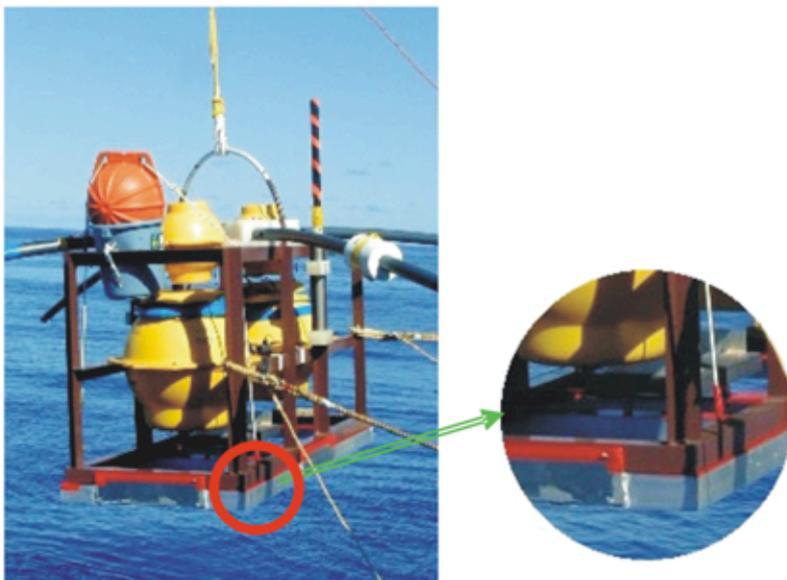
**Figure 4-3-2.** Recovery buoy-rope system. The stopper is fixed between lead weight and OBEM aluminum frame. Once the lead weight is released, the stopper becomes free and the buoy rises ahead of the OBEM body.
