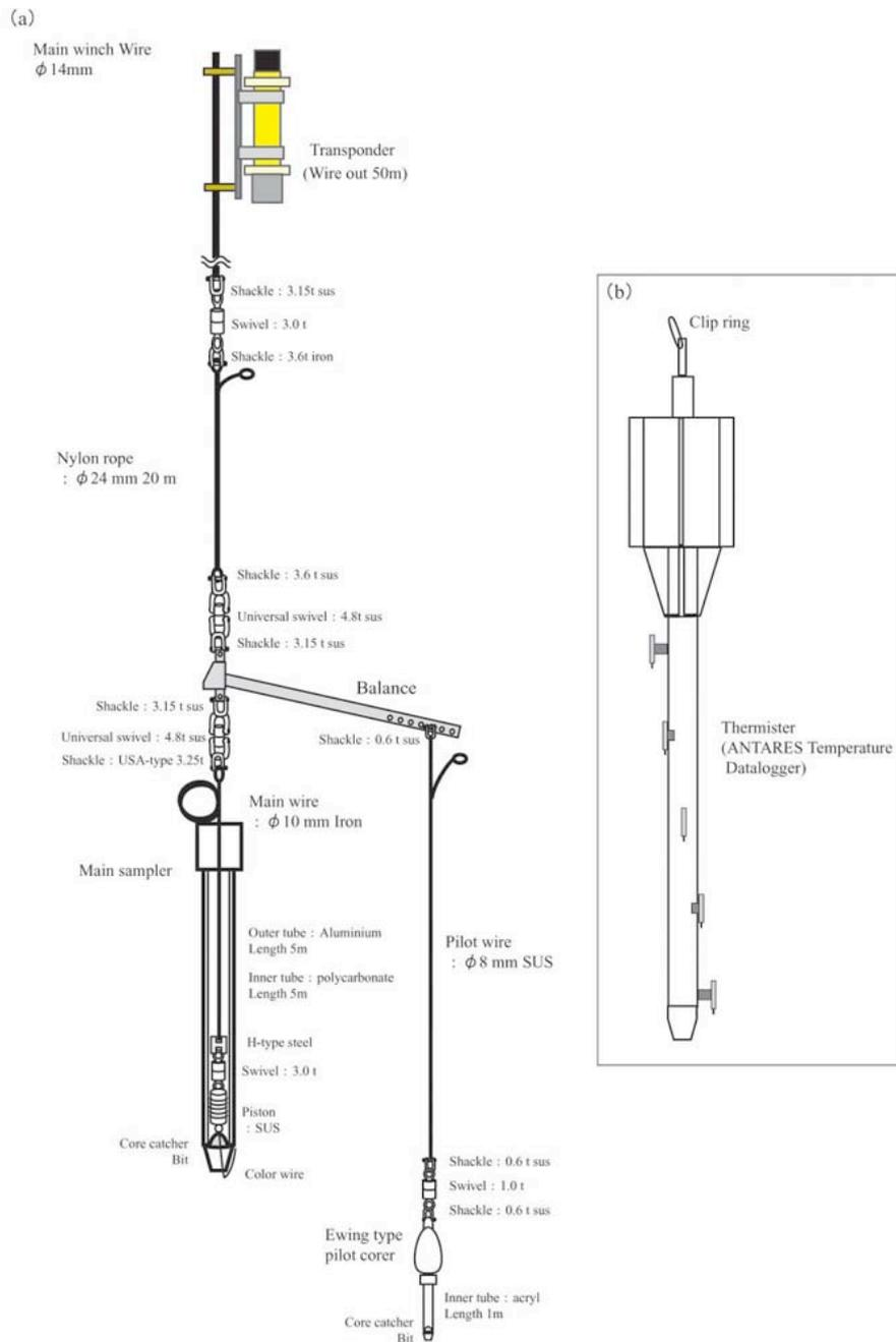
(a)Piston corer system, (b)Position of five Thermisters
