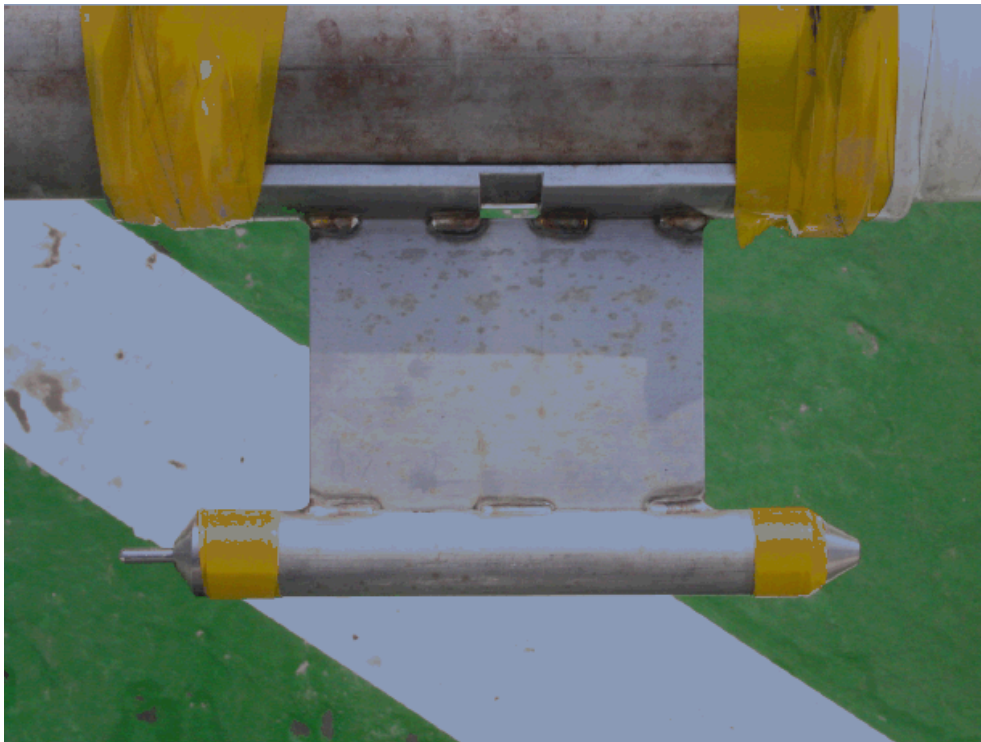
Photo 4-4-1.2. Miniaturized Temperature Data Logger (ANTARES Datensysteme GmbH)
