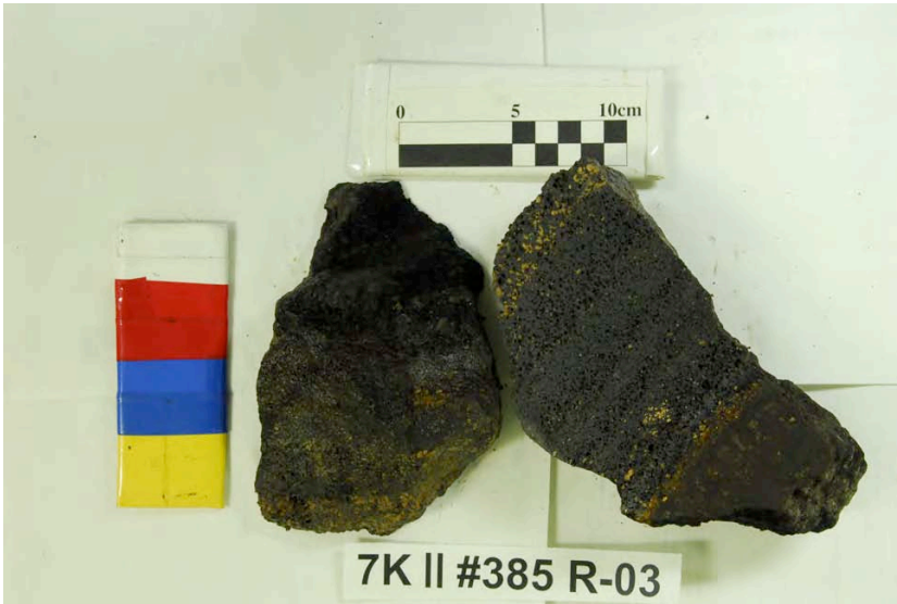
Figure 4-6.12. Basaltic lava sample with thick Mn crust. (7KII #385 R-03)
