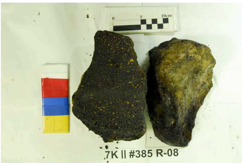
Figure 4-6.14. Basaltic lava sample containing relatively large amount of mafic minerals such as olivine, orthopyroxene and clinopyroxene (?). (7KII #385 R-08)
