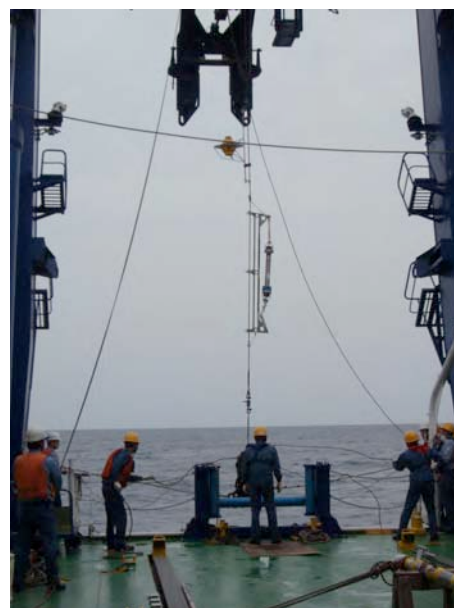
Photo 4-2.2. The acoustic relay system.
