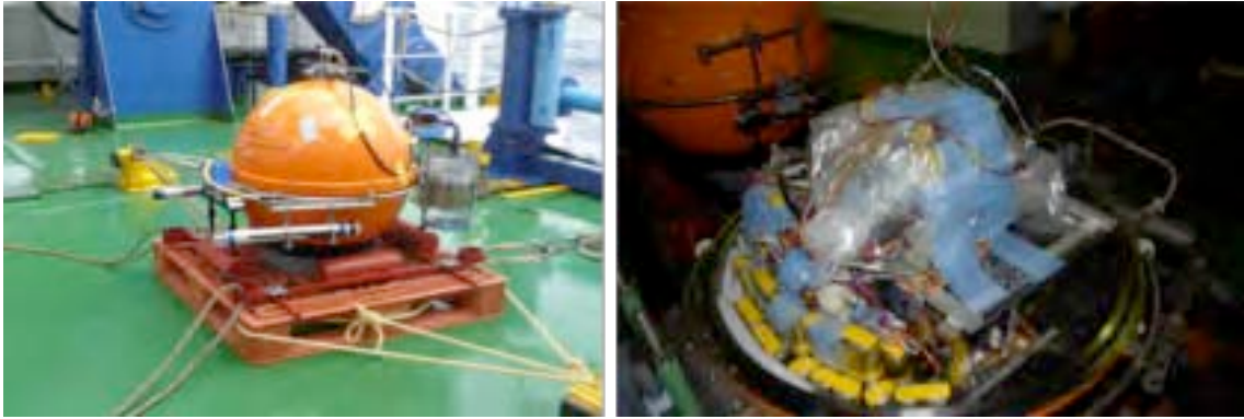
Photo 4-3.1. Appearance (left) and inside (right) of BBOBS. See to above text for detail description.
