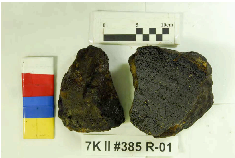
Figure 4-6.13. Basaltic lava sample with vesicle layers. (7KII #385 R-01)
