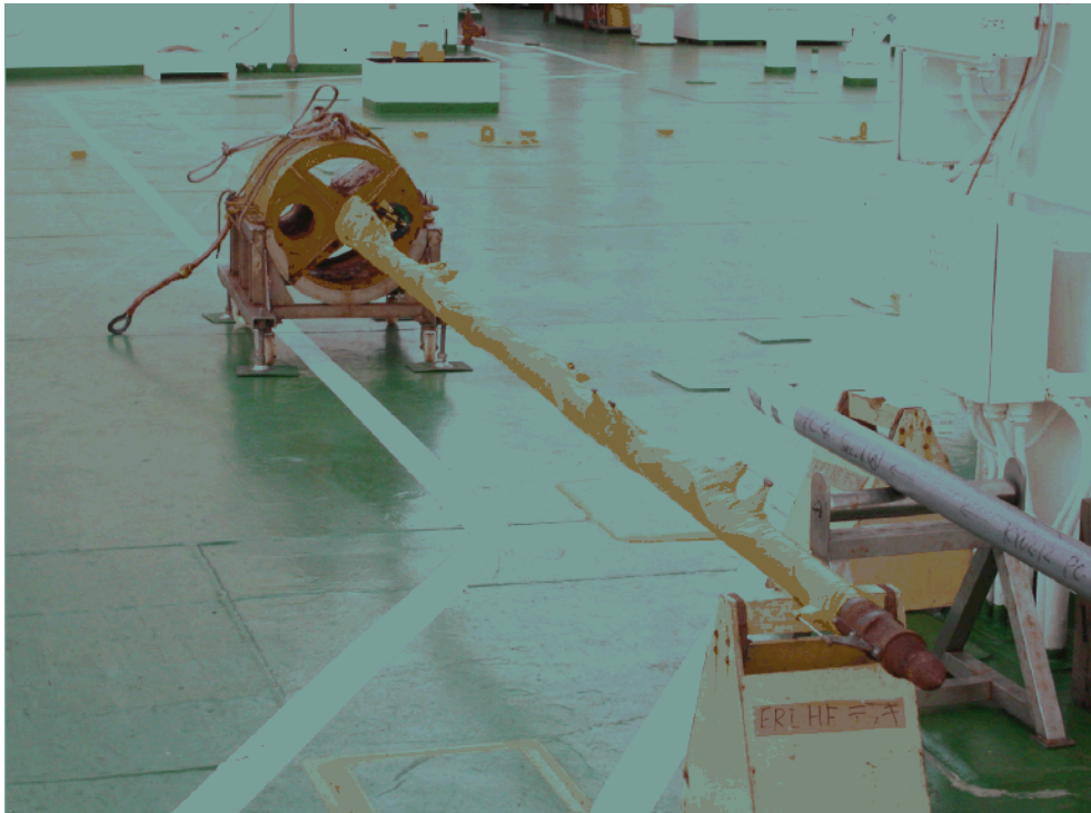
Photo 4-4-1.1. Deep-sea heat flow probe with Ewing type temperature sensors.
