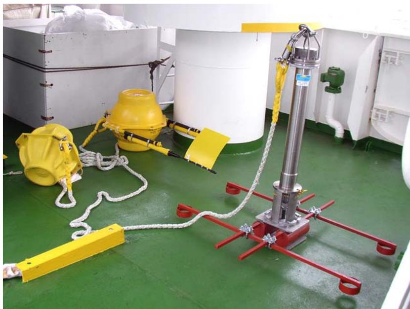
Figure. 3.4-9. Pop-up water temperature measurement system (PWT).
