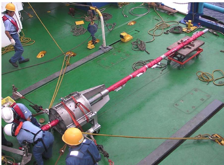
Figure.4-4. HFPC with compact temperature data loggers (MTLs).
