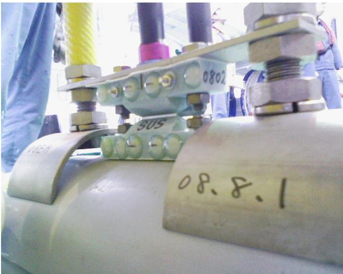
Fig. 3.4-14. Releasing unit. A stainless plate (SUS), connecting the glass sphere and the weight, is cut after receiving an acoustic command.
