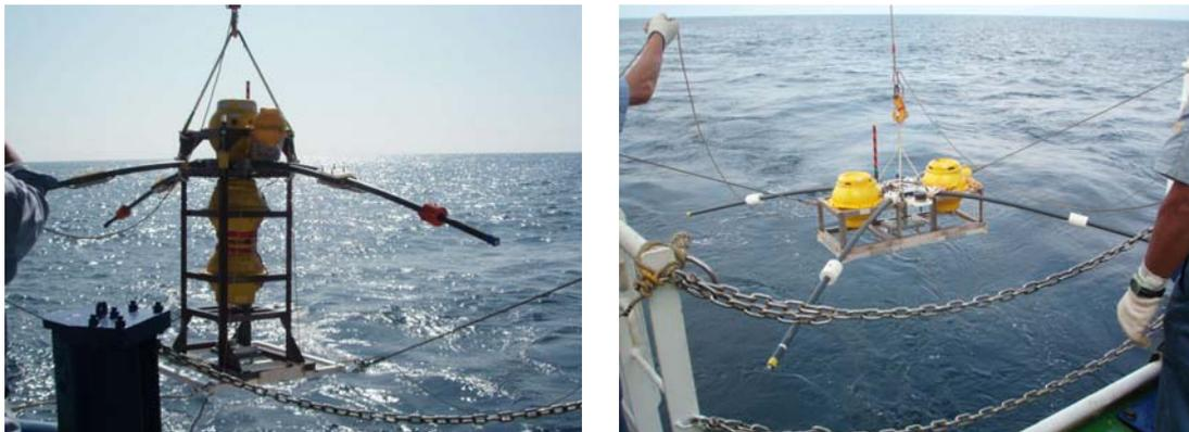
Figure 3.4-15. Type 1 LT-OBEM (left) and Type 2 LT-OBEM (right).
