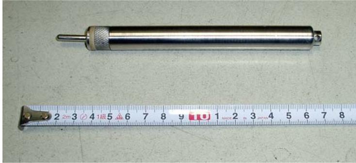
Figure 3.4-2. ANTARES Miniaturized Temperature Data Logger (MTL).
