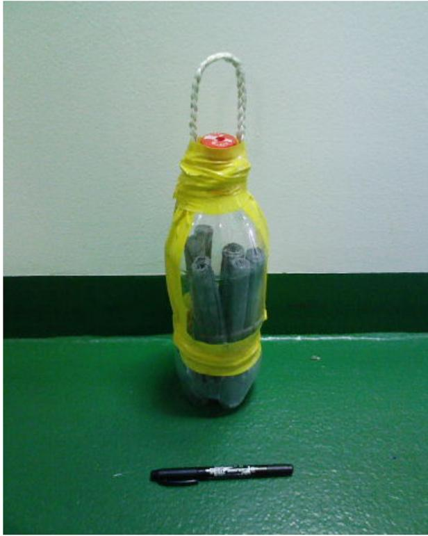
Figure 3.4-19. (f) Sinker at the end of cable
