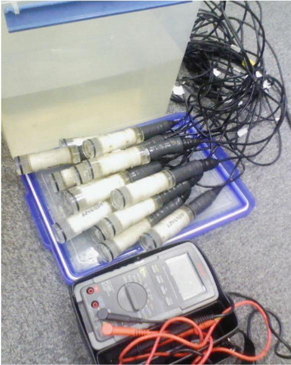
Figure 3.4-13. Ag-AgCl electrodes. They are normally soaked in the salt water tank, and checked with measuring the voltage differences between electrodes.
