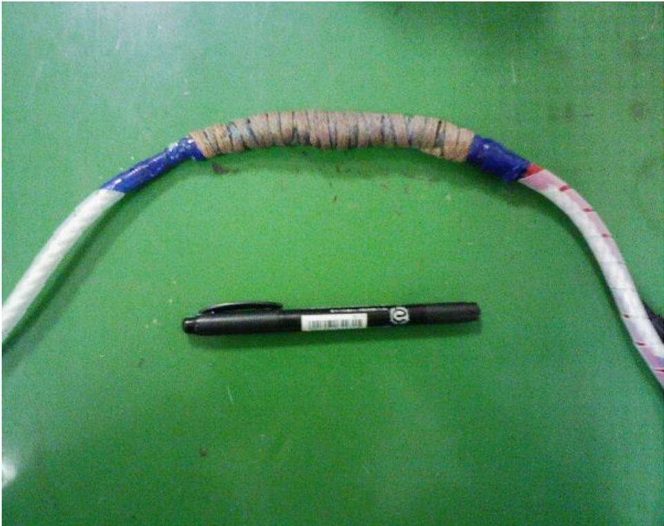
Figure 3.4-19. (e) Receiver electrode (upper) and source electrode (lower).
