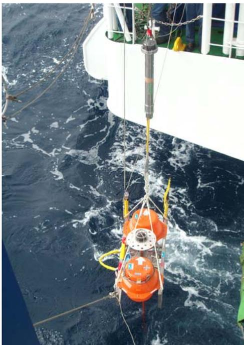
Figure 3.5-1. Deployment of a pop-up heat flow instrument (PHF).
