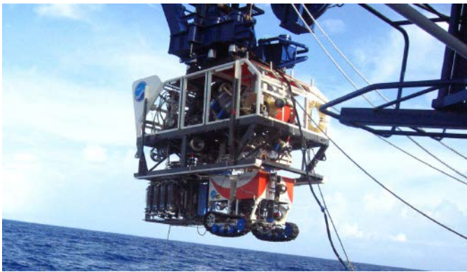
Fig. 1 The automatic bottom inspection and sampling mobile ABISMO.
