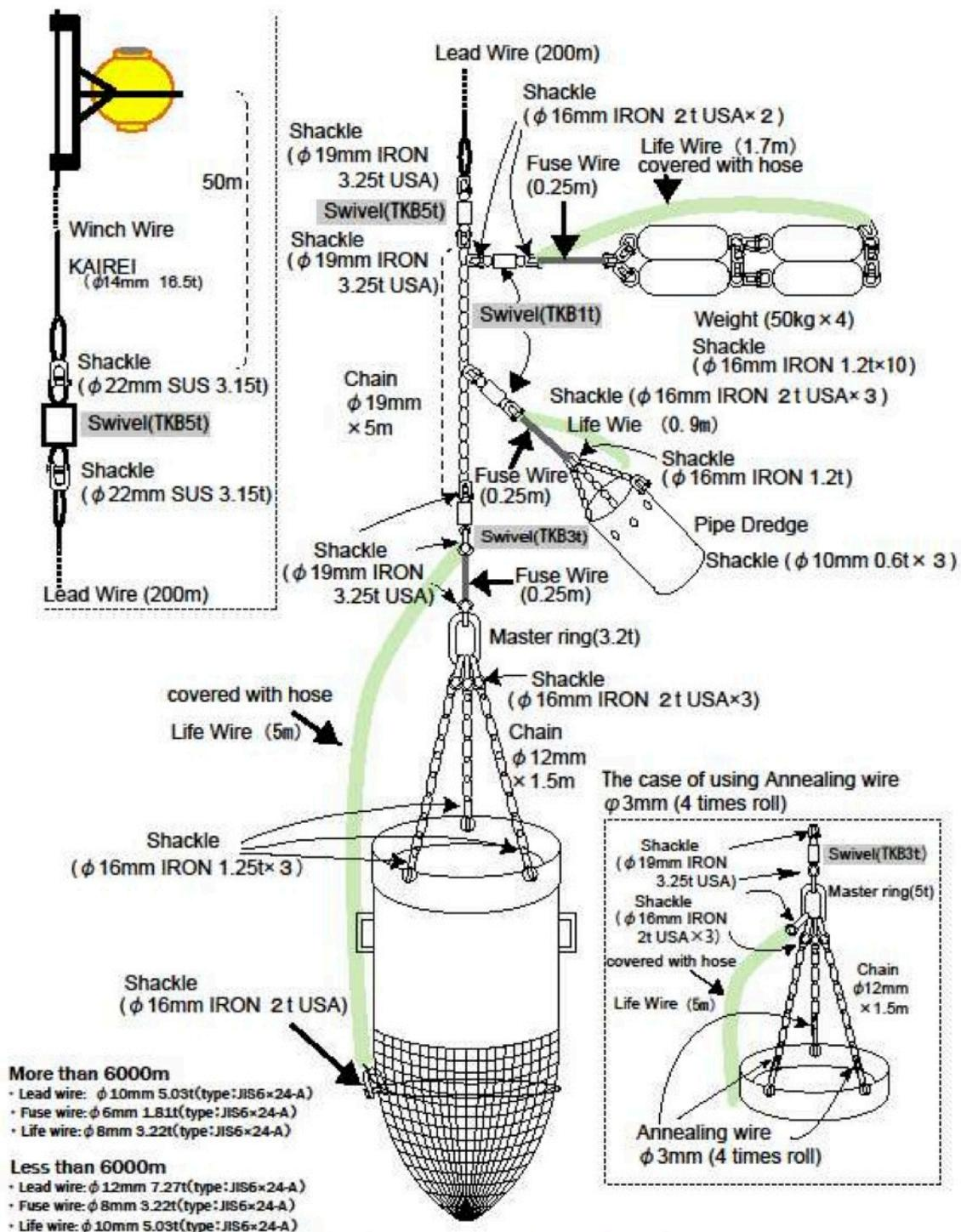
Figure 4. Dredge system with a cylinder-shape dredge.
