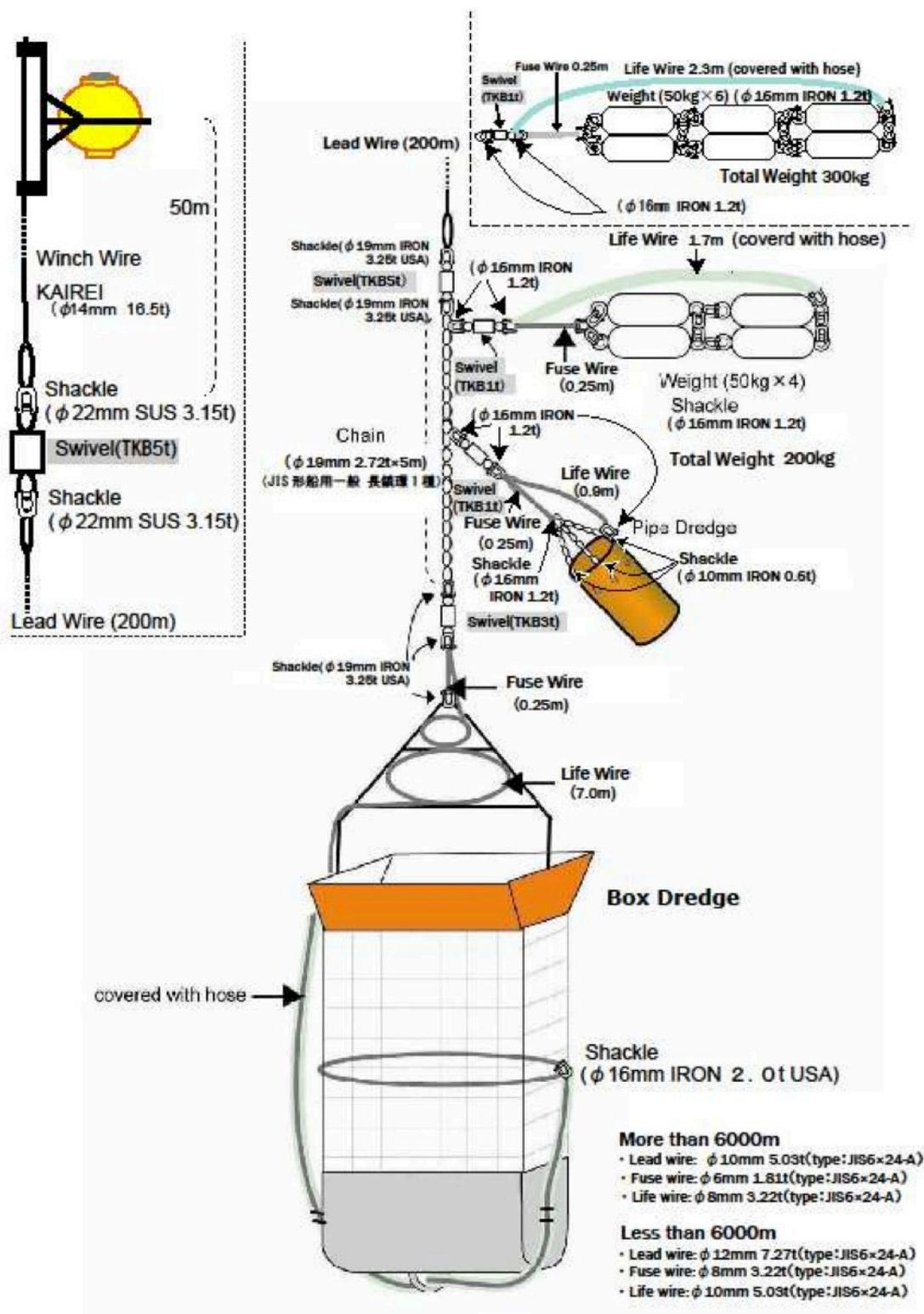
Figure 3. Dredge system with a box-shape dredge.
