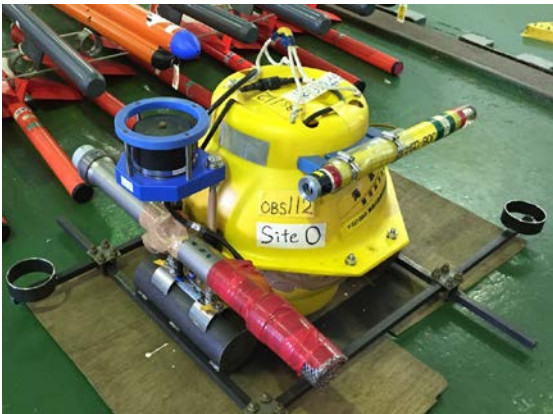
Fig.6-3-5 OBS with KDC transponder.
