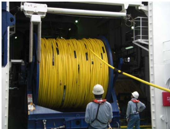
Figure 6-2-2 Streamer cable and winch.
