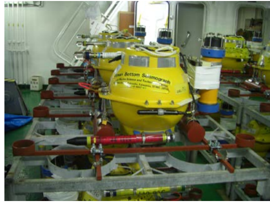
Fig.6-3-6: OBS with SGK transponder.
