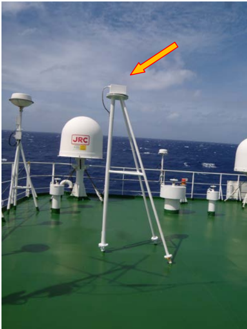
Figure 6-8-1 Magnetic sensor (Deck) Figure 6-8-2 Measurement unit (upper) and Data recording unit (lower)
