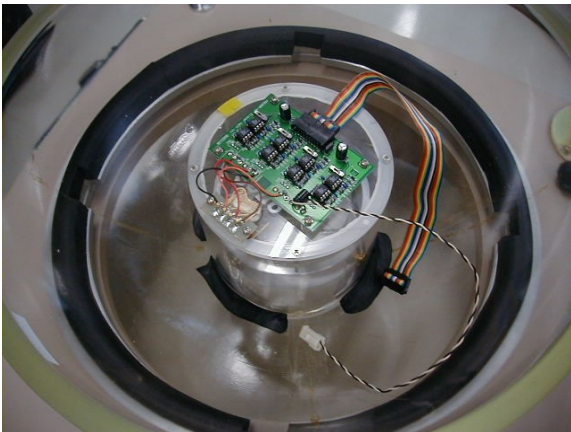
Fig. 6-3-2: OBS sensors in glass sphere. Fig. 6-3-3: OBS recorder and battery.
