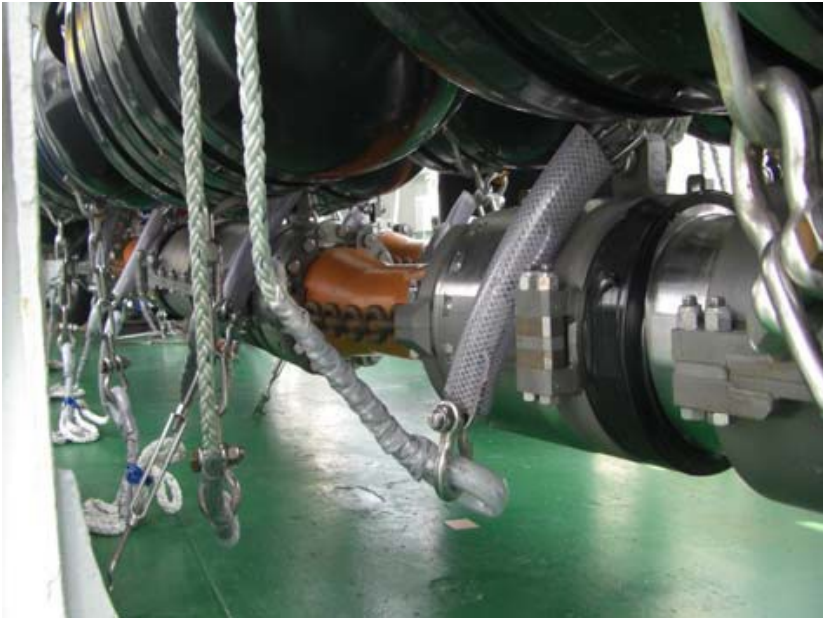
Fig. 6-1-1: APG airgun on deck.
