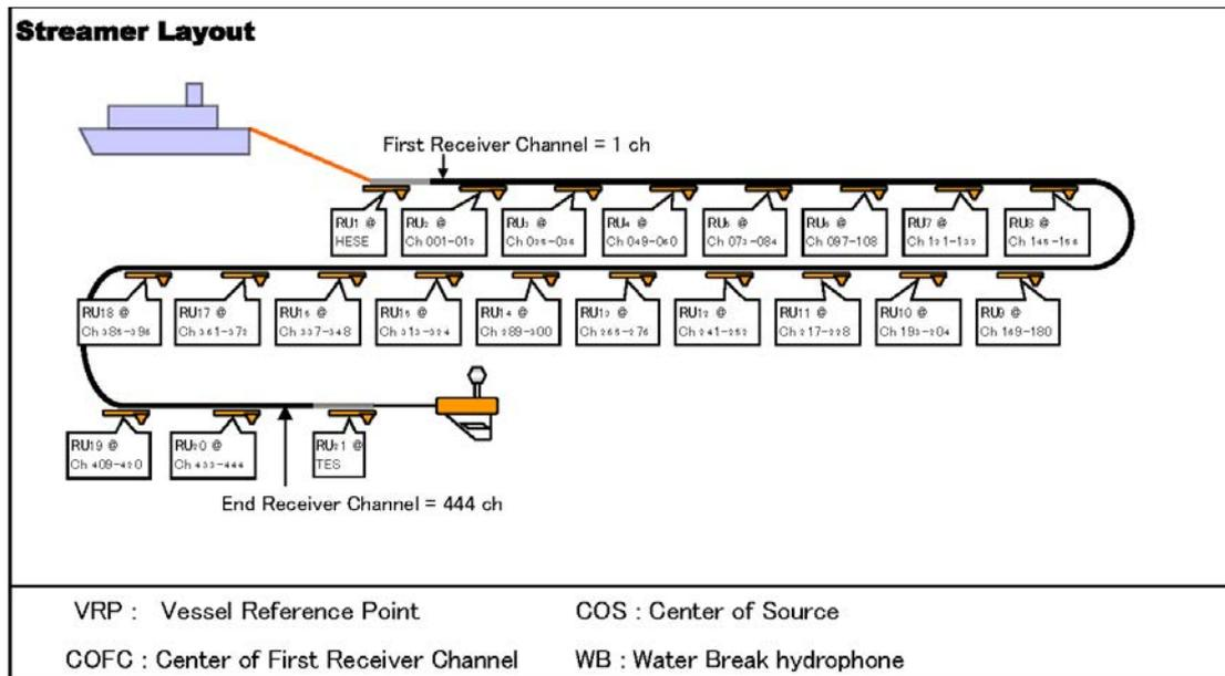
Fig. 4: Streamer cable configuration during the MCS survey.
