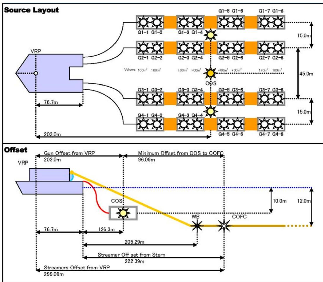
Fig. 3: Vessel towing geometry during the MCS survey. Top figure shows the source (airgun system) layout, bottom figure represents source–receiver depth and position, and navigation offsets.
