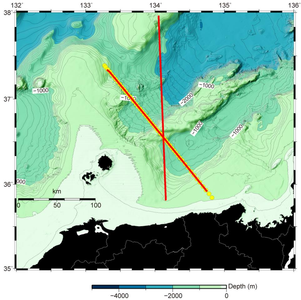
Fig. 10: Map of the bathymetry around the survey area and seismic survey lines in this cruise. Red lines and yellow circles show the MCS lines and positions of deployed OBSs, respectively.
