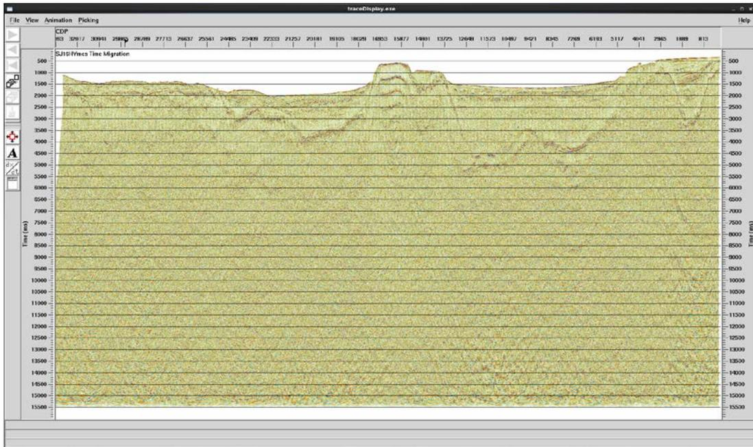
Fig. 5: Example of MCS profile with onboard processing (SJ16HY line).
