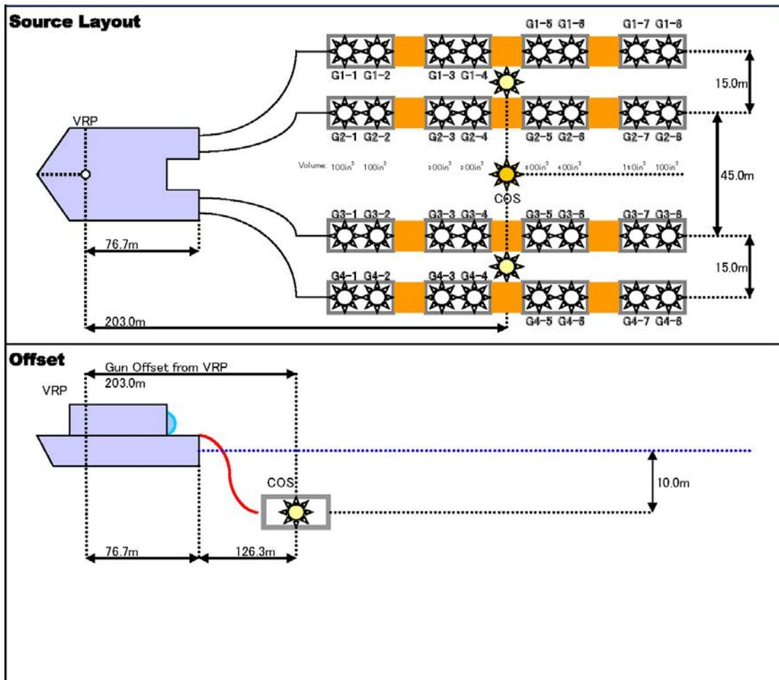
Fig. 7: Vessel towing geometry during the seismic refraction survey on the SJ16HY line. Top figure shows the source (airgun system) layout, bottom figure represents source depth and position, and navigation offsets.
