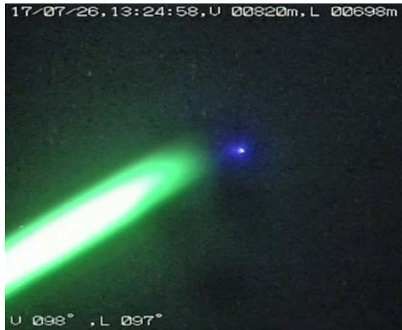
Fig. 2 blue light like a star was carrier light from the vehicle, and green light like a jet was carrier light from the launcher.
