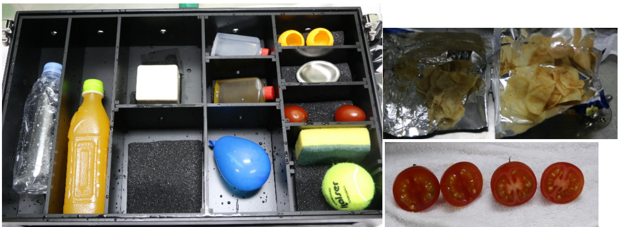
After diving. Empty plastic bottle, balloon and tennis ball returned to the original (filled with the air) but hollow stainless steel soap and ping-pong balls were broken by water pressure.
