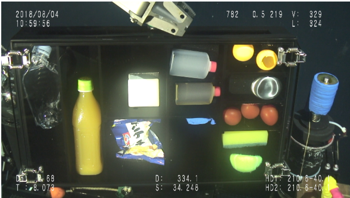
A part of submarine experiments. From left, empty plastic bottle, orange juice filled plastic bottle, tofu (soy bean curd), snack food, water filled and oil filled plastic small bottle, balloon, ping-pong balls, hollow stainless steel soap, tomatoes, sponge and tennis ball under high pressure of 334m depth.
