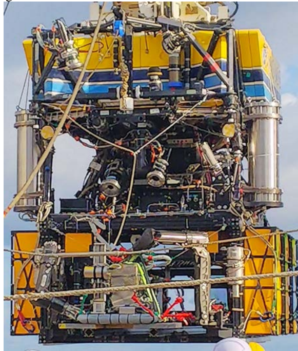
Fig.4-1 the Mobile Pressure Calibrator with the ROV Hyper Dolphin
