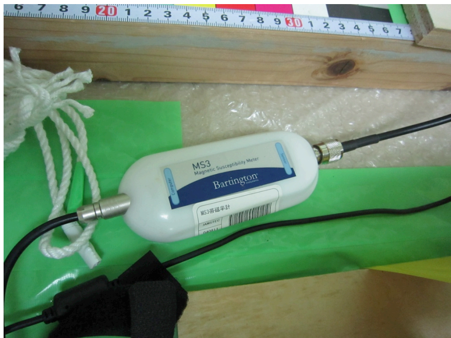
Fig. 6.1.2-2. Close up photograph of the magnetic susceptibility meter Model MS3 (Bartington Instruments Ltd.)
