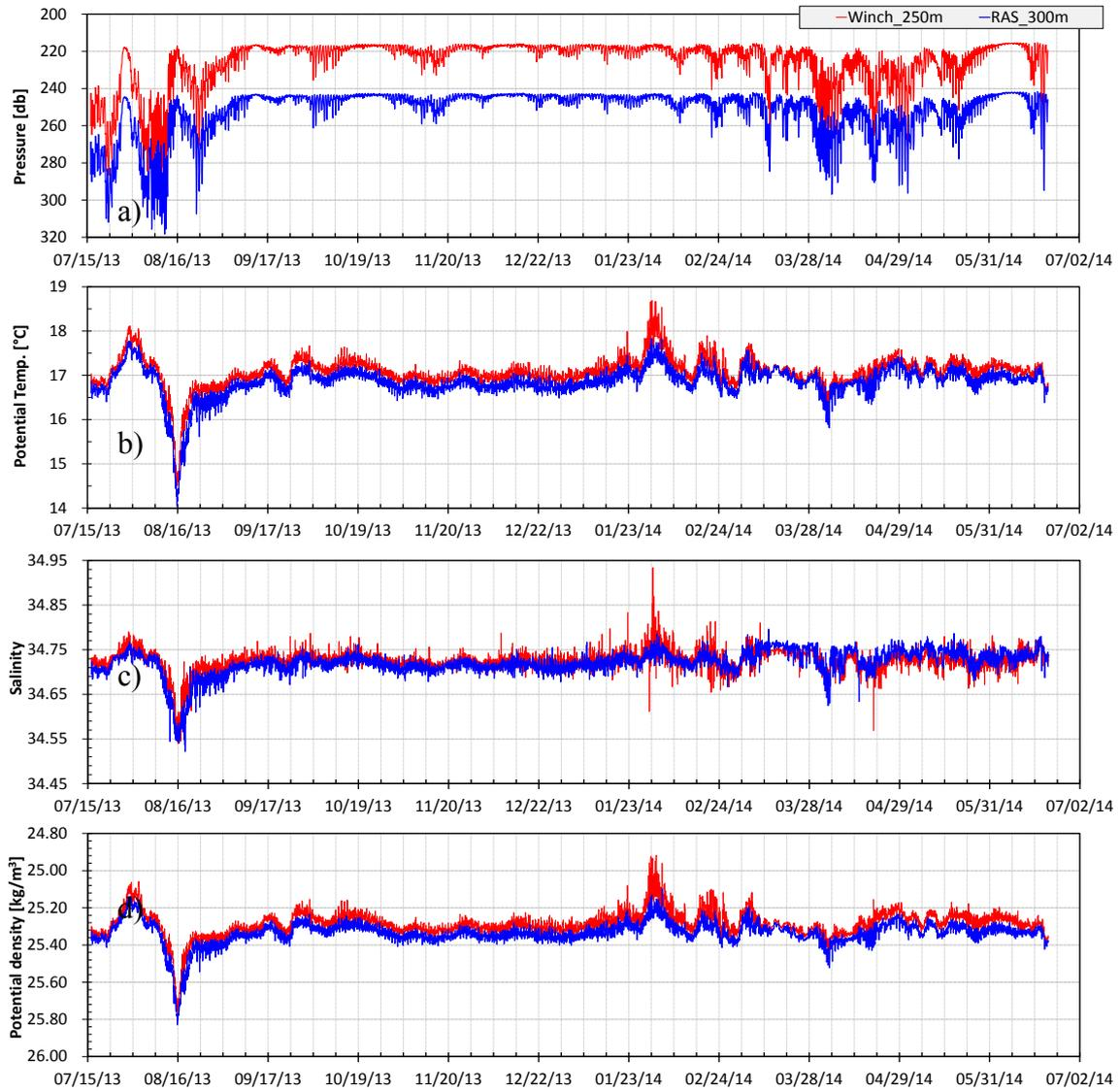
Figure 13. Pressure (a), potential temperature (b), Salinity (c) and potential density at the Winch and RAS during the deployment.
