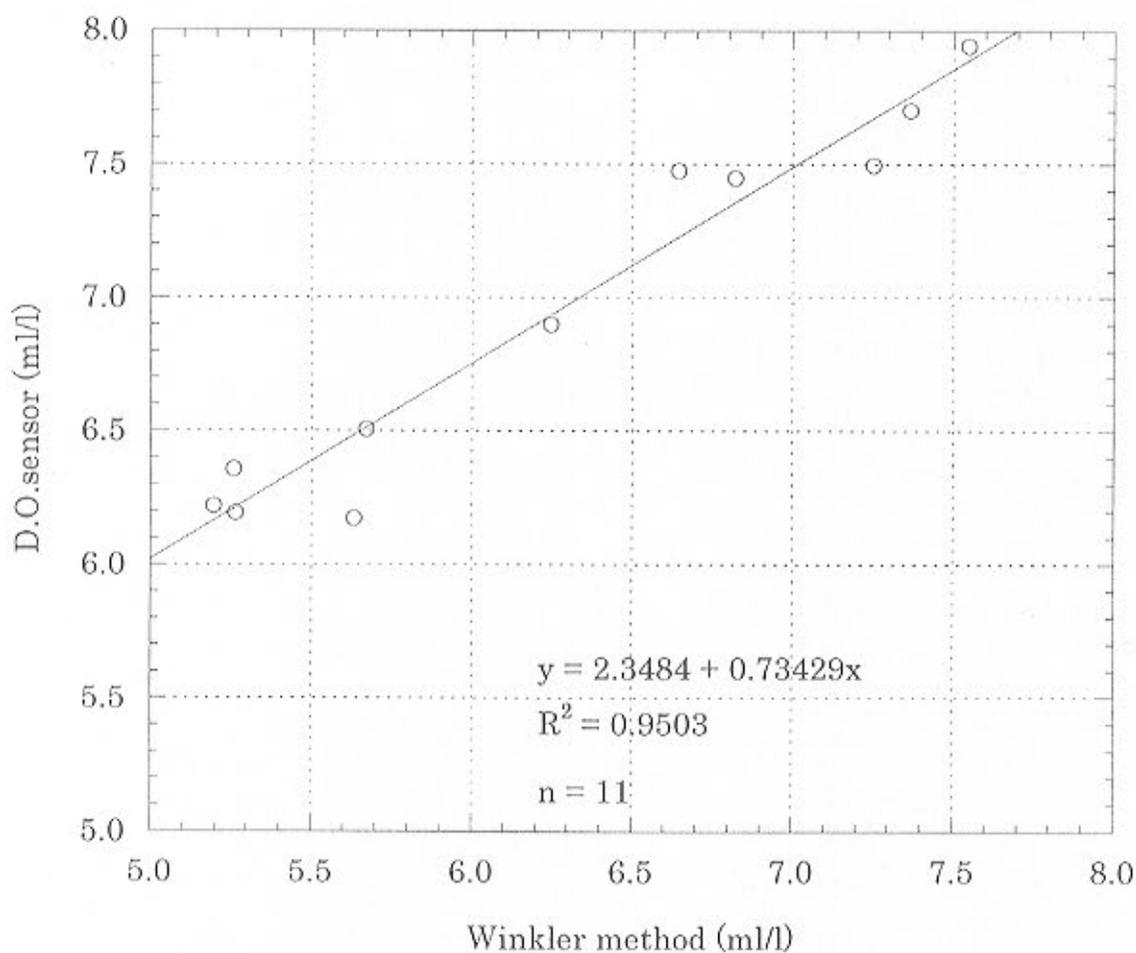
Fig.3.17.3-2 Comparison between the D.O. value measured by D.O. sensor of the Sea Surface Monitoring System and by Winkler method for 11 samples obtained during MR00-K01 cruise.
