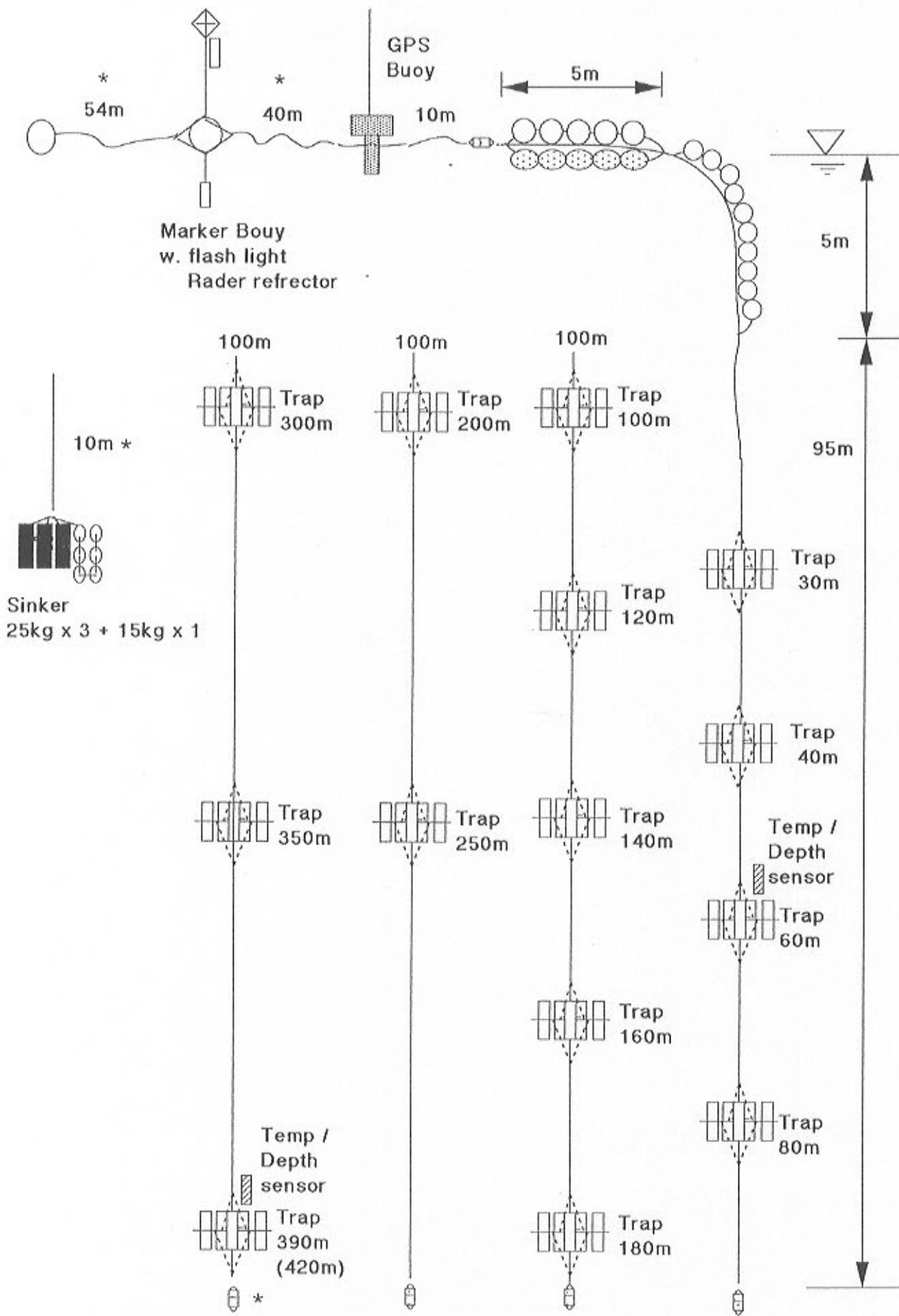
Fig. 3.12.1 Drifting sediment trap mooring system by JAMSTEC
