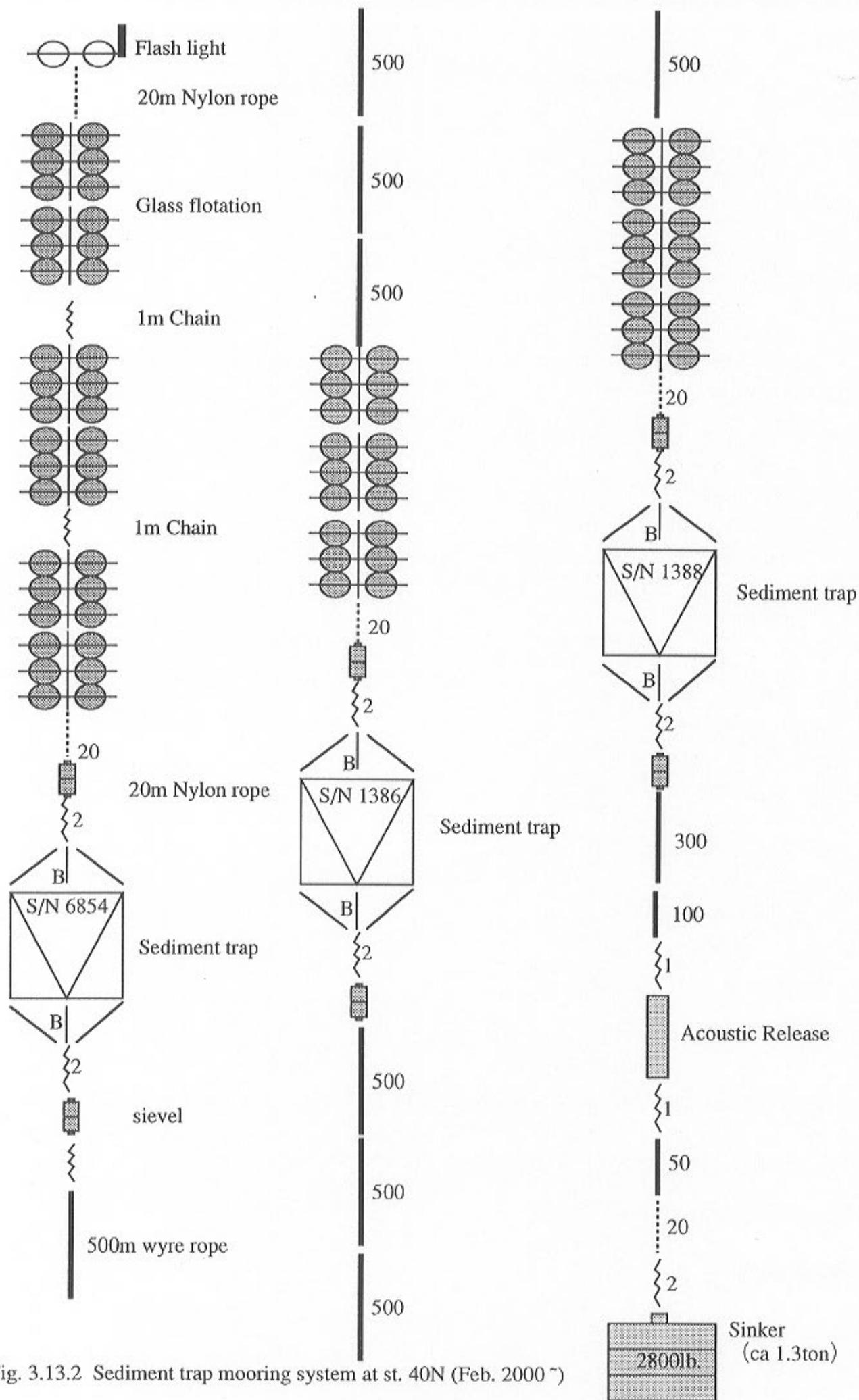
Fig. 3.13.2 Sediment trap mooring system at st. 40N (Feb. 2000 ~)
