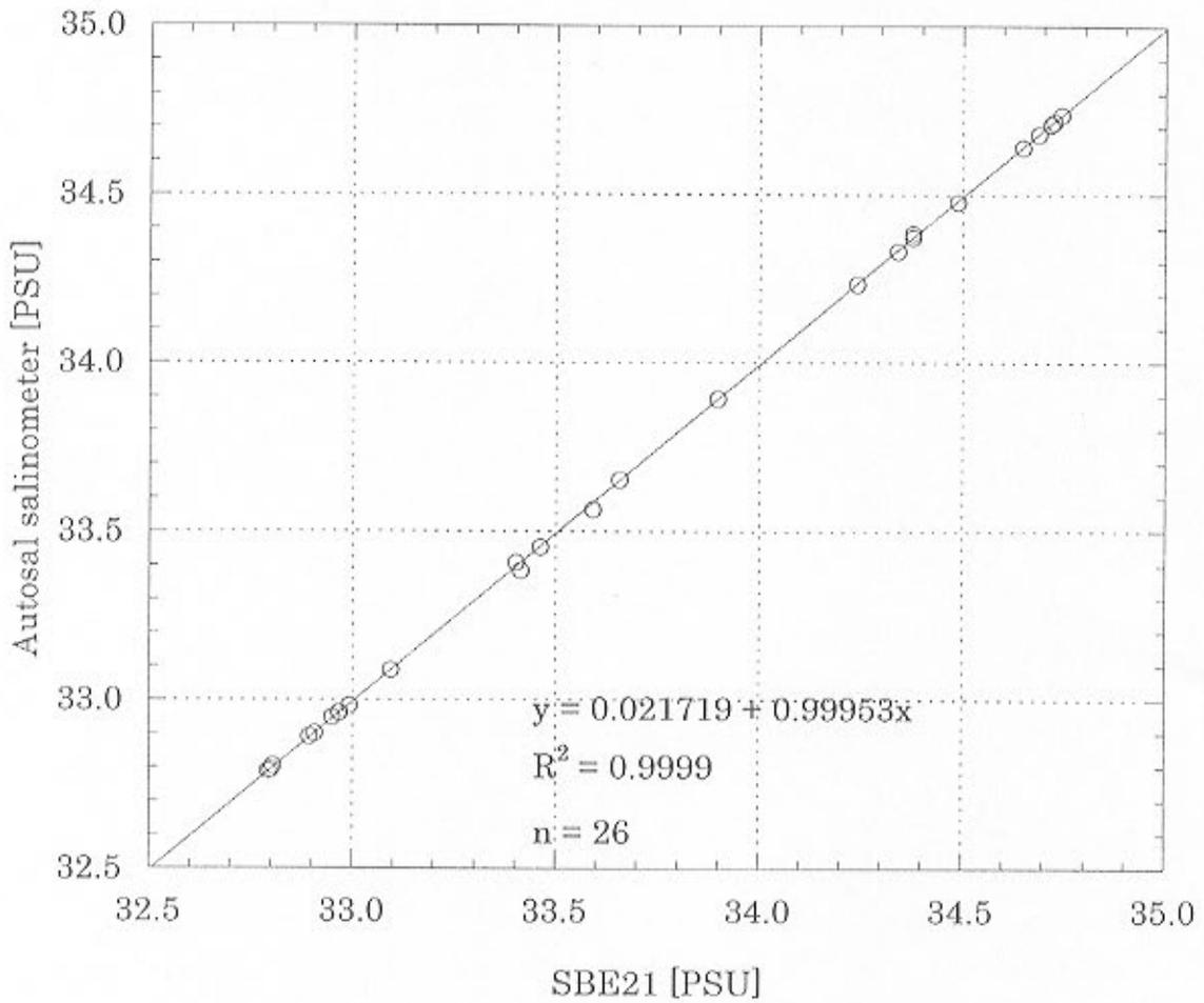
Fig. 3.17.3-1 Comparison between the salinity values measured by SBE21 of the Sea Surface Monitoring System and Autosol salinometer for 26 samples. Note: Salinity in this figure is not corrected.
