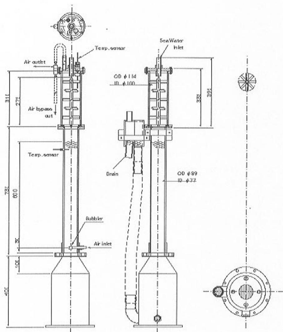
Fig. 1 Schematic of Tandem equilibrator
