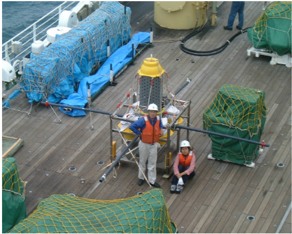
Figure 1. SeaFloor ElectroMagnetic Station before deployment
