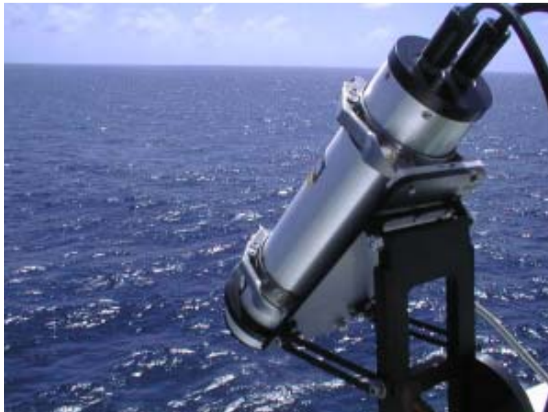
Figure 6. SAS radiance L_t sensor
