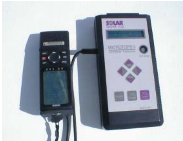
Figure 9. Microtops II hand-held sunphotometer
