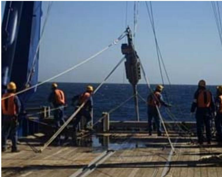
**Picture – 2 launching the piston corer at station 1**
