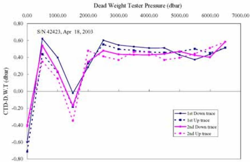
**Fig.3.1.3.1: The residual pressures between the Dead Weight Tester and the CTD.**
