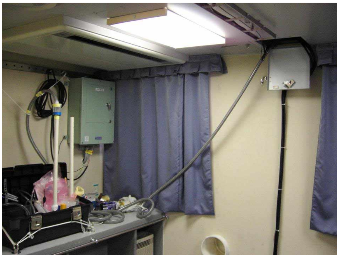
Figure 3. Atmospheric laboratory equipment set-up. The intake line was routed from its location atop ship, through a wiring portal and into the laboratory. The image shows the intake hose attached to the filter funnel/manifold/pump set-up as a sample was being collected.
