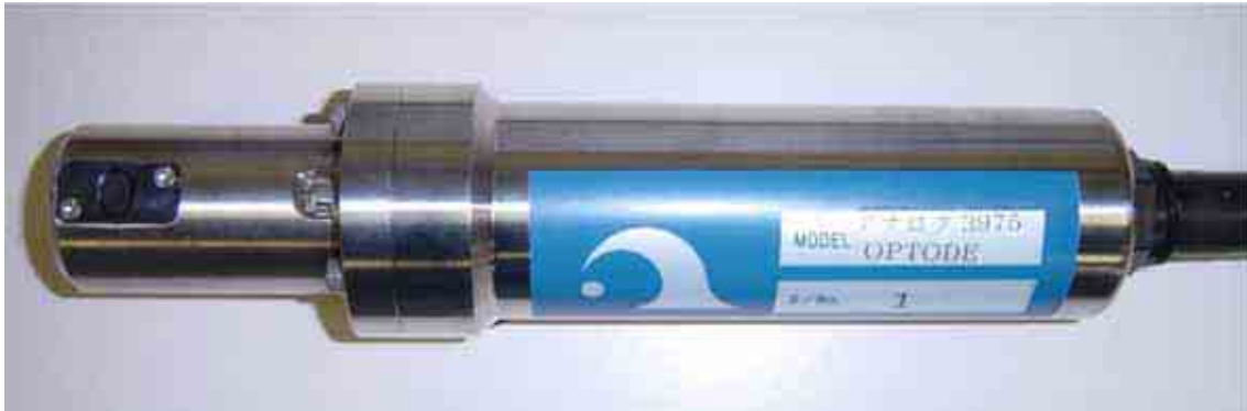
Figure 3.1.3.5. Aanderaa Oxygen Optode (3830) with analog adaptor (3966). The analog adaptor is packed into titanium housing made by Alec Electronics, Japan.
