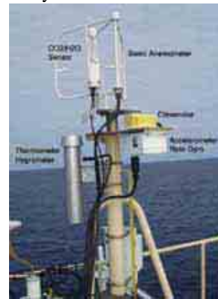
Fig. 2.1.3-1 Turbulent flux measurement system on the top deck of the foremast.
