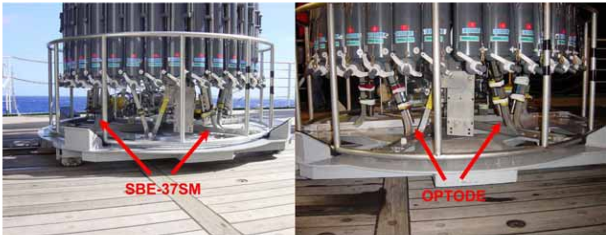
Figure 4.2.3.1. Photos of the moored CTDs and oxygen sensors attached to the CTD/RMS frame.
