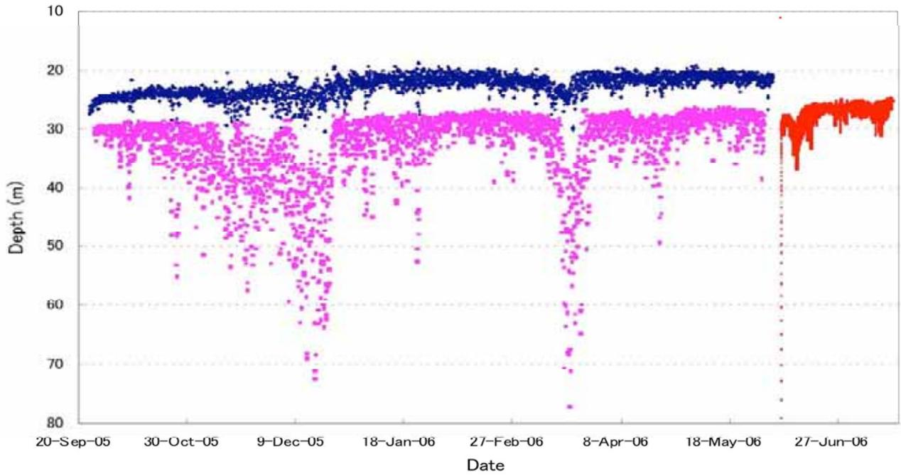
Fig 3.1.4-11 Top Buoy depth by Depth sensor
