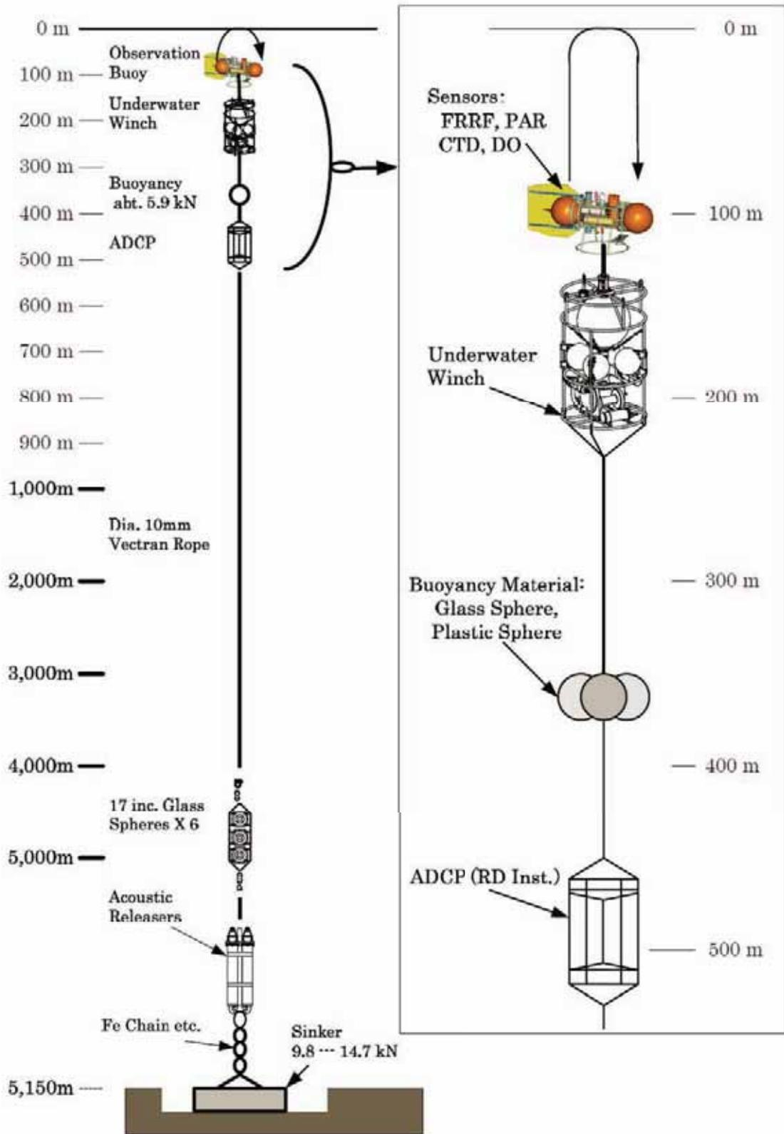
Fig. 1a. Schematic diagram of the POPPS Mooring.
