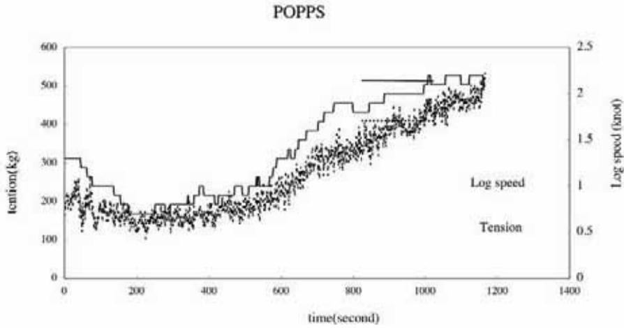
Fig6.1-6 Correlation coefficient of rope tension/ship's speed in deployment at k2 station
