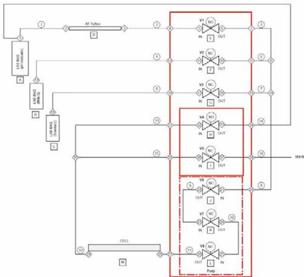
Fig. 2.9.2-1 Flow diagram of the CO<sub>2</sub> sensor.
