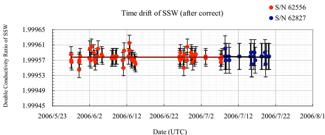
**Fig. 2.2.2.2 the history of double conductivity ratio of the Standard Seawater batch P146 of serial number 62556 and 62827 (after correct)**
