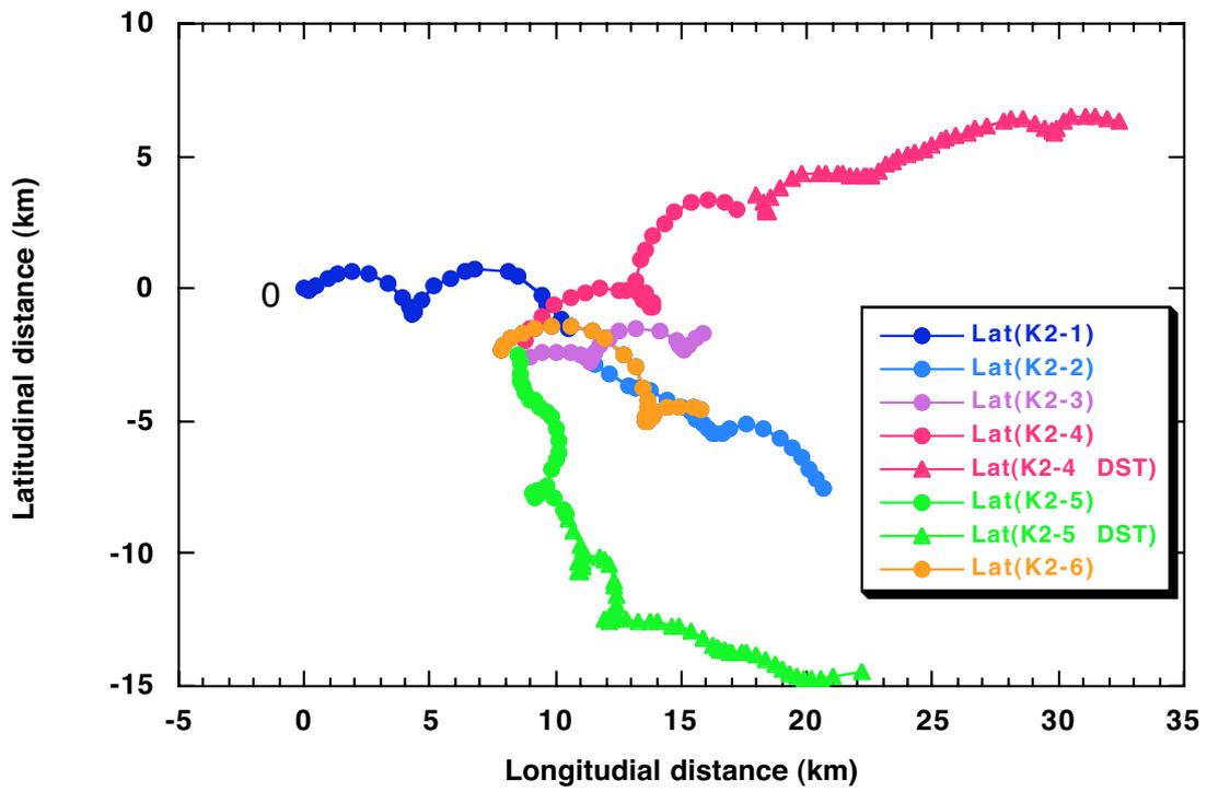
Fig. 3.5.1.2 Track of drifter (GPS buoy) for 6 deployments. Position 0 is the point that the drifting mooring system was deployed at the first time.
