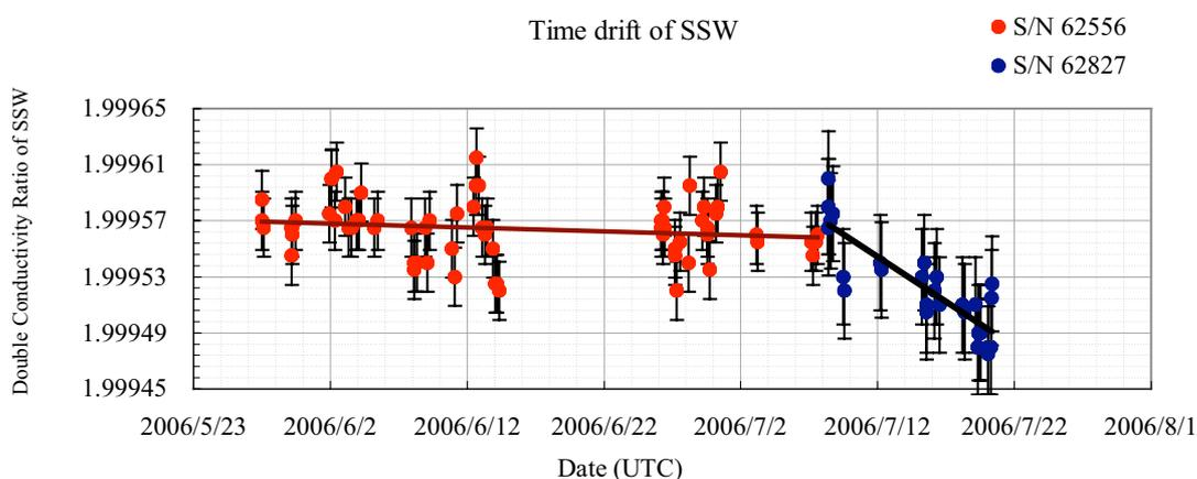
**Fig. 2.2.2.1 the history of double conductivity ratio of the Standard Seawater batch P146 of serial number 62556 and 62827**
