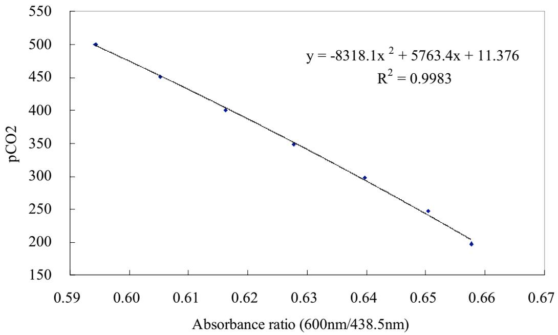
Fig. 2.9.2-3 Calibration curve of TB solution.
