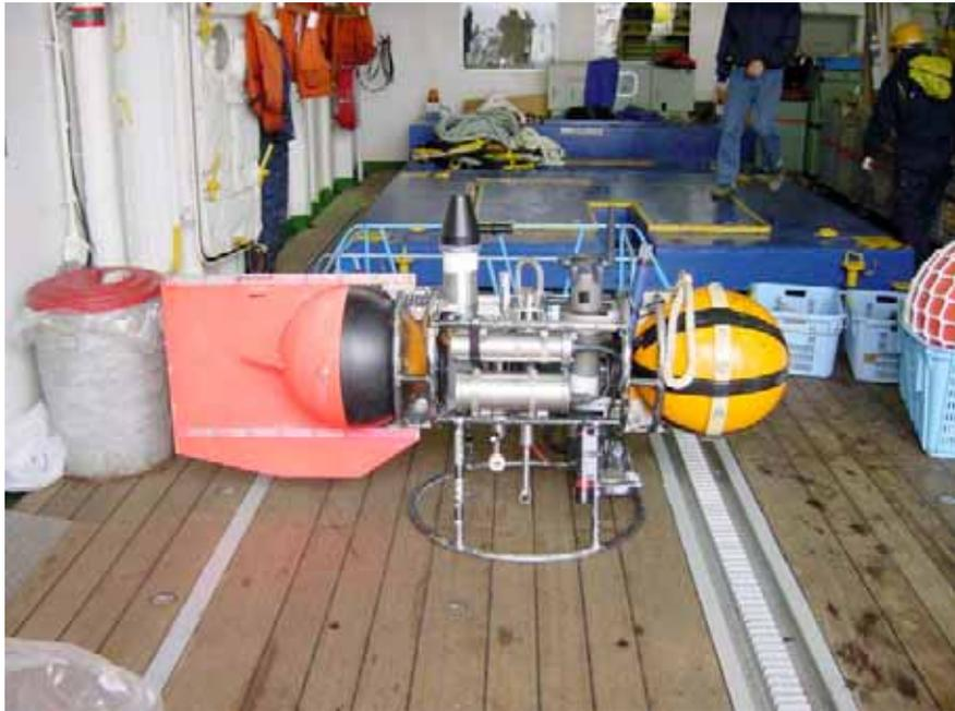
Fig. 1c. The observation buoy equipped with the FRR fluorometer.
