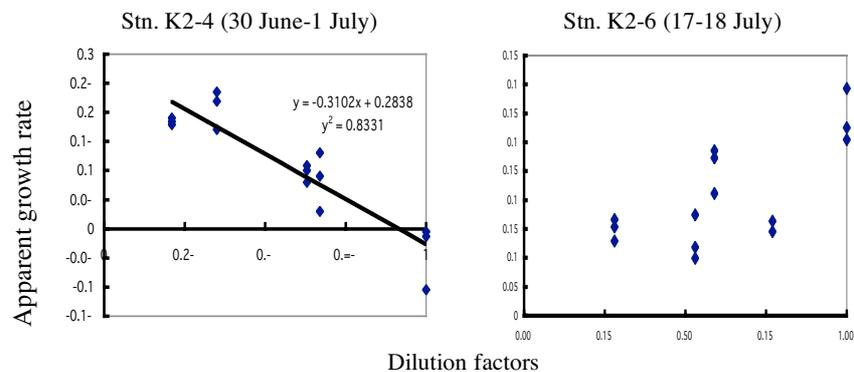
Theoretically, negative correlation between apparent phytoplankton growth rates and dilution factors is shown like a graph of Stn. K2-4 (30<sup>th</sup> June ~ 1<sup>st</sup> July). In this experiment, ‘true’ phytoplankton growth rate and grazing coefficient of microzooplankton were estimated at 0.28 d<sup>-1</sup> and 0.31 d<sup>-1</sup>, respectively. However, some experiments failed like a result of Stn. K2-6, the negative correlation is not recognized.
