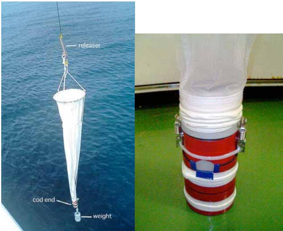
Fig. 3: NORPAC net used for sampling (left) and protected cod end (right)
