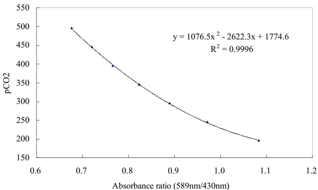
Fig. 2.9.2-2 Calibration curve of BCP solution.
