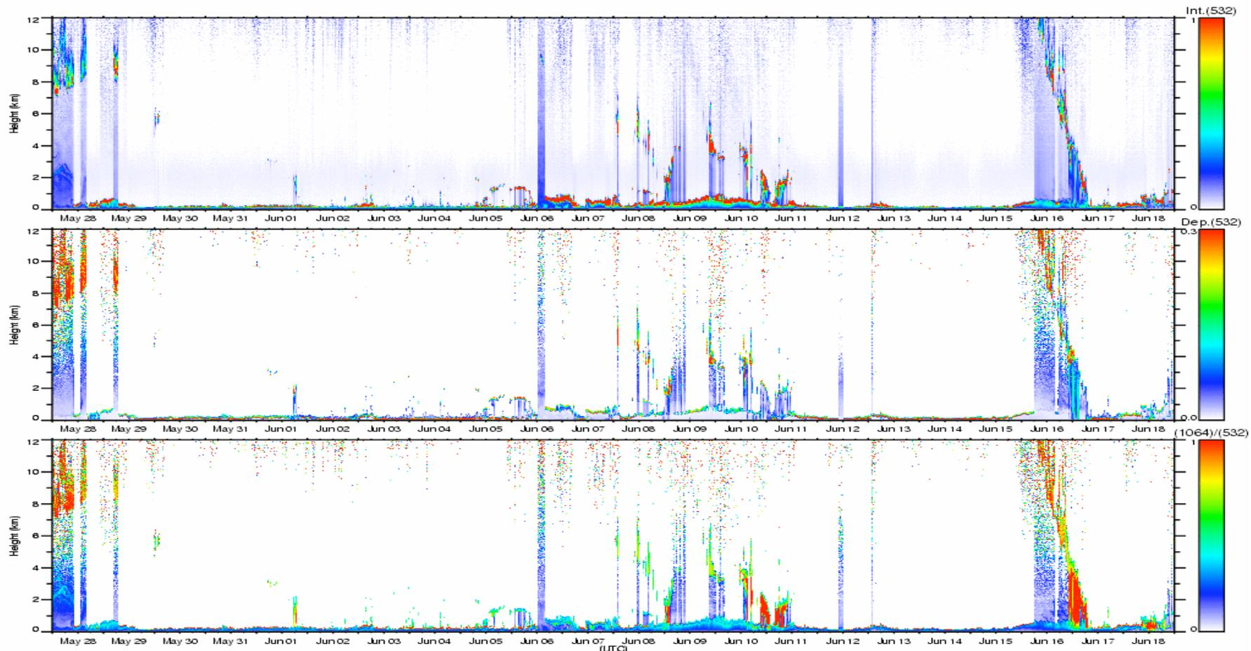
Figure 1 Time-height indications of backscattering intensity at 532 nm (top), depolarization ratio at 532 nm (middle), and ratio of backscattering intensities between 1064 nm and 532 nm (bottom), during MR06-03 leg 1. Depolarization ratio is a measure of non-sphericity of particles, and ratio of two wavelengths is a measure of particle size.
