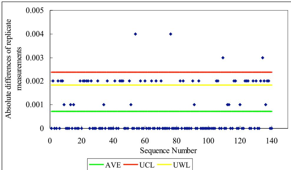
Figure 2.6-1 Range control chart of the absolute differences of replicate measurements carried out in the analysis of pH during the MR06-03 cruise.
