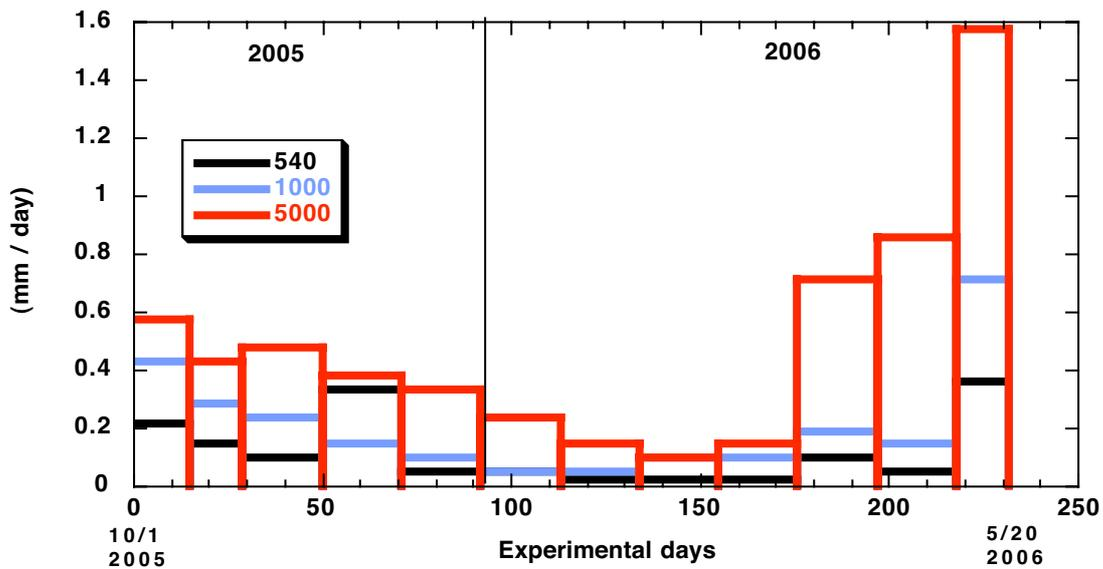
Fig. 3.1.4.3.1 Total mass flux at 540 m, 1000 m and 5000 m between October 2005 and May 2006
