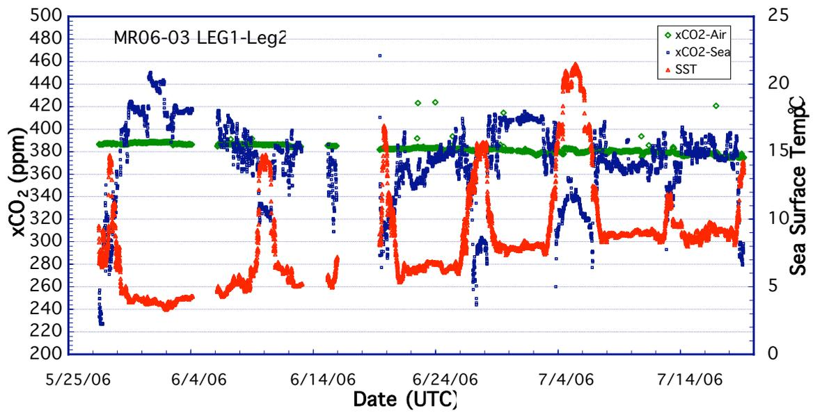
Figure 2.9.1 Mole fraction of CO<sub>2</sub> (xCO<sub>2</sub>) in atmosphere (green) and surface seawater (blue), and SST (red) that was analyzed in the North Pacific during MR06-03 cruise.
