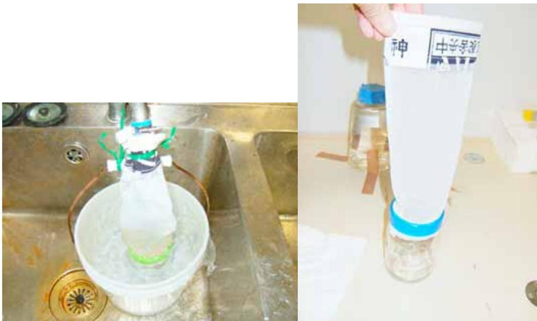
Fig. 4: Surface water filtration (left) and the filtration apparatus(right)
