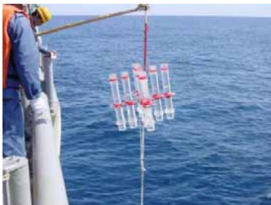
Photo 3.5.3.1 Drifting Sediment Trap
