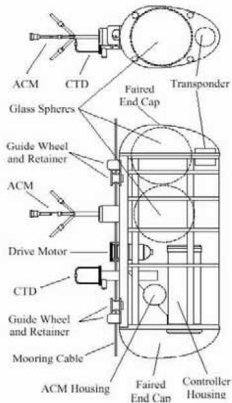
Fig.3.1.2-1 Cut away side and top views of the MMP showing the major components of the system. The overall dimensions of the faired external shell are 124 cm \* 51 cm\* 34 cm
