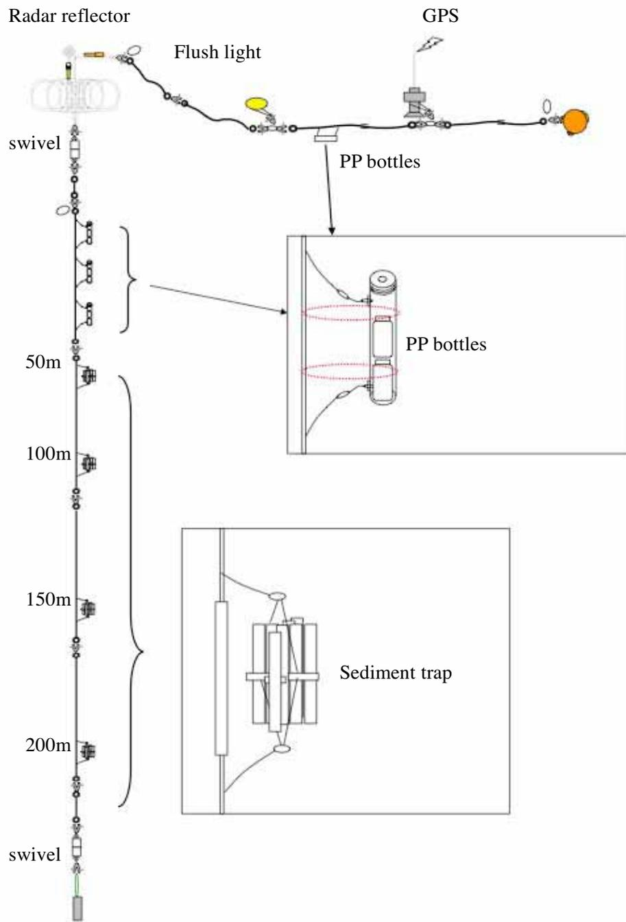
Fig. 3.5.1.1 Drifting mooring system
