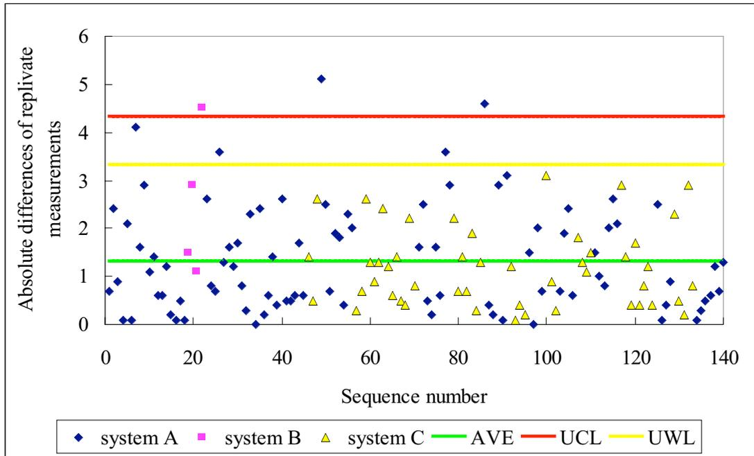
Figure 2.7.-1 Range control chart of the absolute differences of replicate measurements carried out in the analysis of DIC during the MR06-03 cruise.
