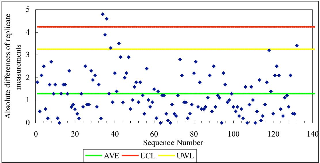
Figure 2.8-1 Range control chart of the absolute differences of replicate measurements carried out in the analysis of TA during the MR06-03 cruise.
