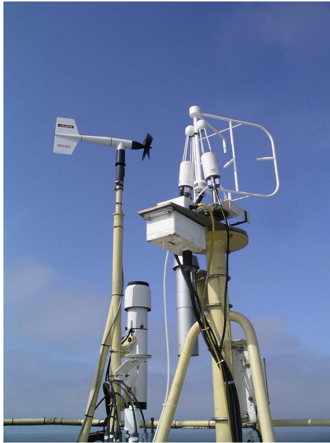
Fig.1. Installation of the turbulent flux and ship motion correction systems on the top of the foremast.
