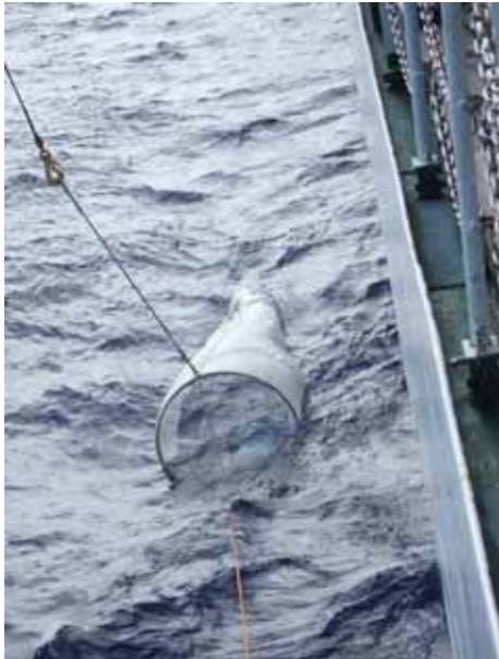
Photo 5.16-2. ORI net trailed on the surface of the western Pacific Ocean on the right side of R/V MIRAI during daytime with a ship speed of 2.5 knot to the sea water.
