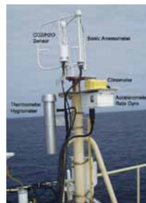
Fig. 5.10-1 Turbulent flux measurement system on the top deck of the foremast.
