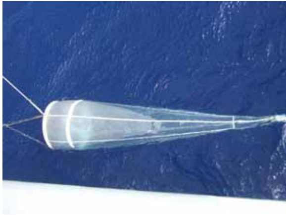
Photo 5.16-1. ORI net trailed on the surface of the western Pacific Ocean on the right side of R/V MIRAI at night with the ship speed of 2.5 knot to the sea water. The net is 6 m long and with diameter of 1.5 m.
