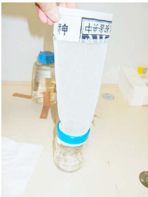
**2-6-fig 1 Surface water filtration apparatus consists of 100  $\mu\text{m}$  opening mesh and glass bottle.**
