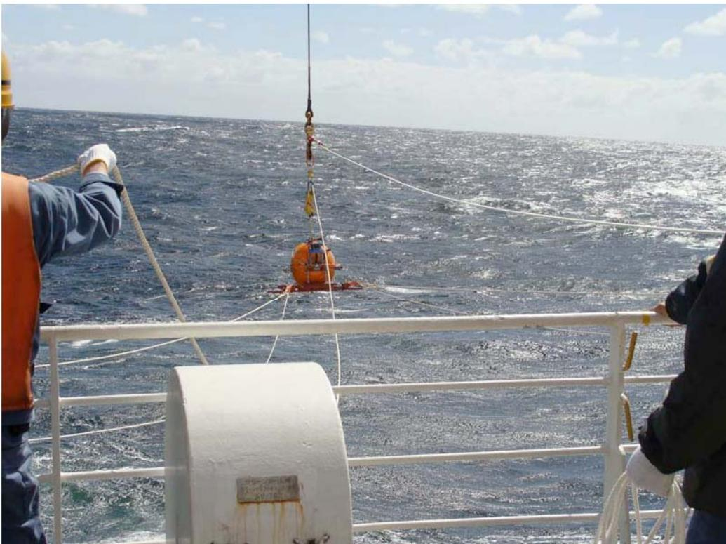
2-4-3-Fig. 2: Deployment work of the LTOBS by the ship crane.
