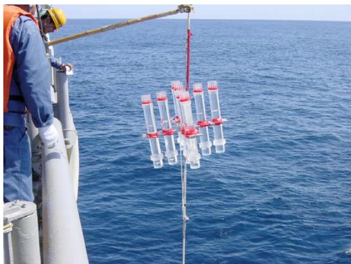
Photo 3.5.2-1 Drifting Sediment Trap.
