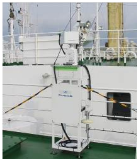
Fig. 7.7.-1. Solar tracker and telescope. The sunlight collected into optical fiber was introduced into the OSA that was installed in an observation room in the
