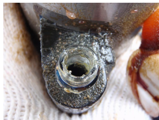
Photo 6 Biofouling state of recovered JES10
