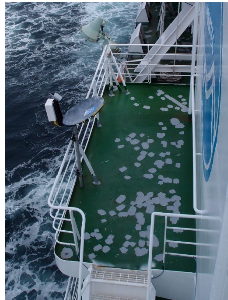
Fig. 2.10.2: The micro rain radar, installed on the starboard side of the anti-rolling tank.
