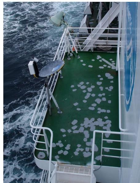
Figure 2.4-2: The micro rain radar, installed on the starboard side of the anti-rolling tank.
