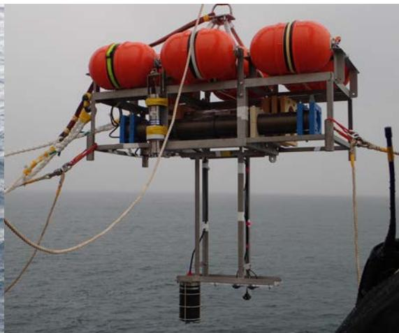
Fig.7 A transceiver for surface station.
