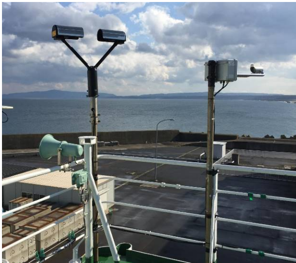
Fig. 4.3.2-1: The two disdrometers (Parsivel and LPM), installed on the roof of the anti-rolling tank.
