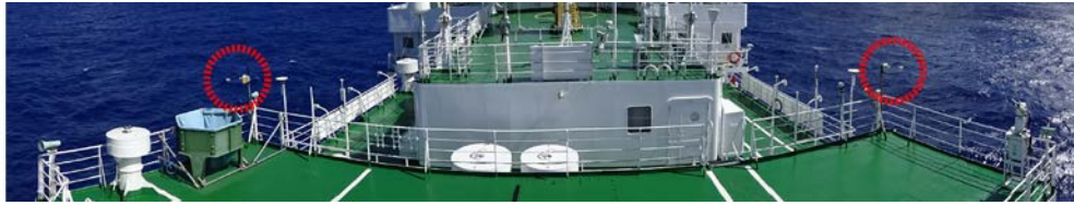
Fig. 5.11-1: The location of the LPM sensors, on the panorama photo looking down toward the bow (from a tower for the radome of the C-band radar). Red broken circle shows the location of LPM sensors.
