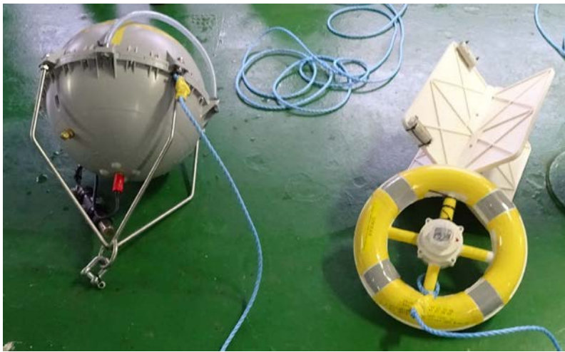
Fig. 5.6-1: The instruments used in the short deployment. Upper panel is for Set 1, consisted of (left) SC40 with CARTHE drogue, (center) Surpact, and (right) CARTHE with DST-CT/CTD. Lower panel for Set 2, consisted of (left) SC40 and (right) CARTHE with DST-CT/CTD.
