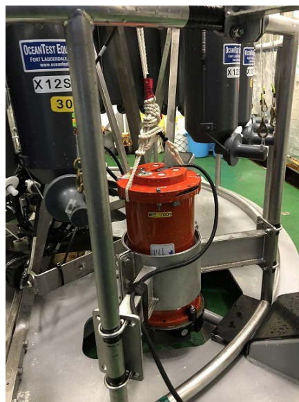
Figure 5.23-1: Mounting of LADCP on CTD System
