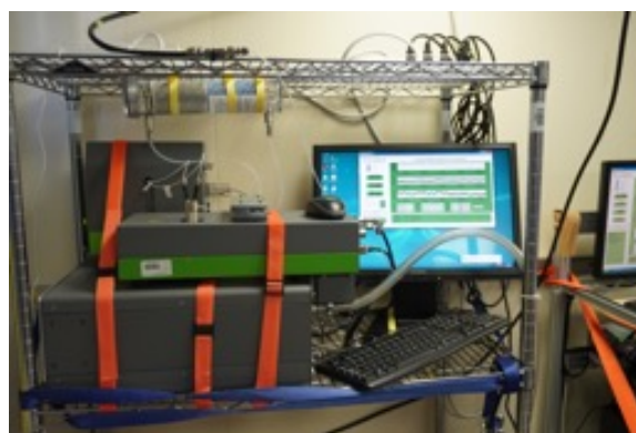
Figure 2.9.1-1: Isotope observing spectrometer system.
