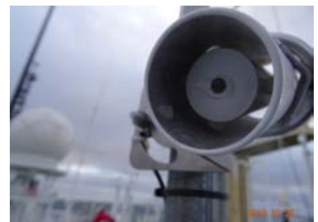
Figure 2.7-7: Example of hard icing just before daily maintenance at 19:36 UTC on 29 October.
