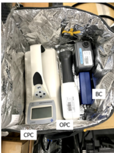
Figure 2.10.2-2: Instruments employed in the tethered-balloon observations.
