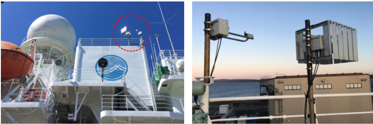
Figure 2.11.1-1: Onboard LPM sensors. (Left) Sensor location indicated by the red broken circle. (Right) Photo of the sensors showing the wind protection “element” mounted on the right-hand (aft) unit.
