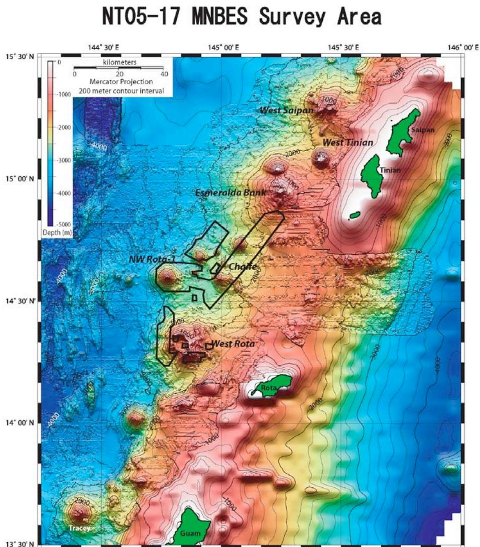
Figure 5.1. Bathymetric map of study area with Seabat survey fields shown by heavy dark lines.
