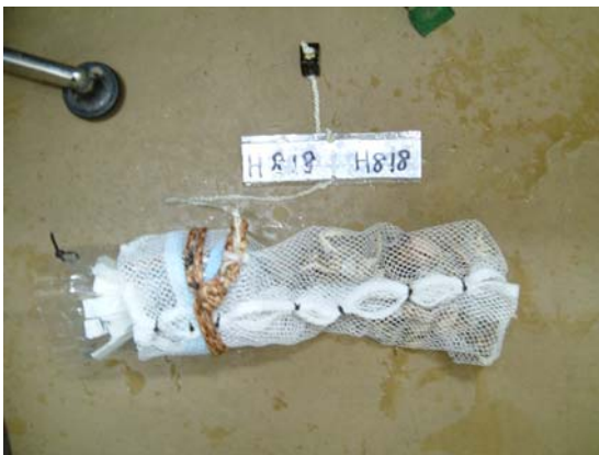
Fig. 22. The bait trap, by which Yunohana crabs are trapped.
