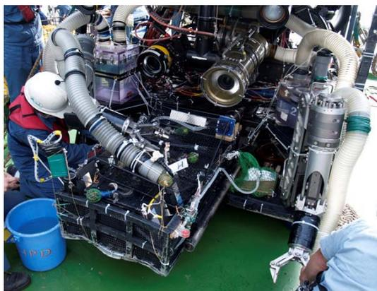
The arrangement of the slurp gun with two nozzle and two canisters
