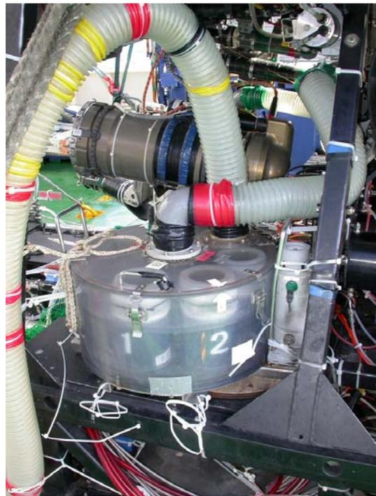
The rotary canister with canister bottles
