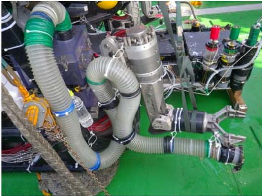
The left nozzle connected to the cubic canister
